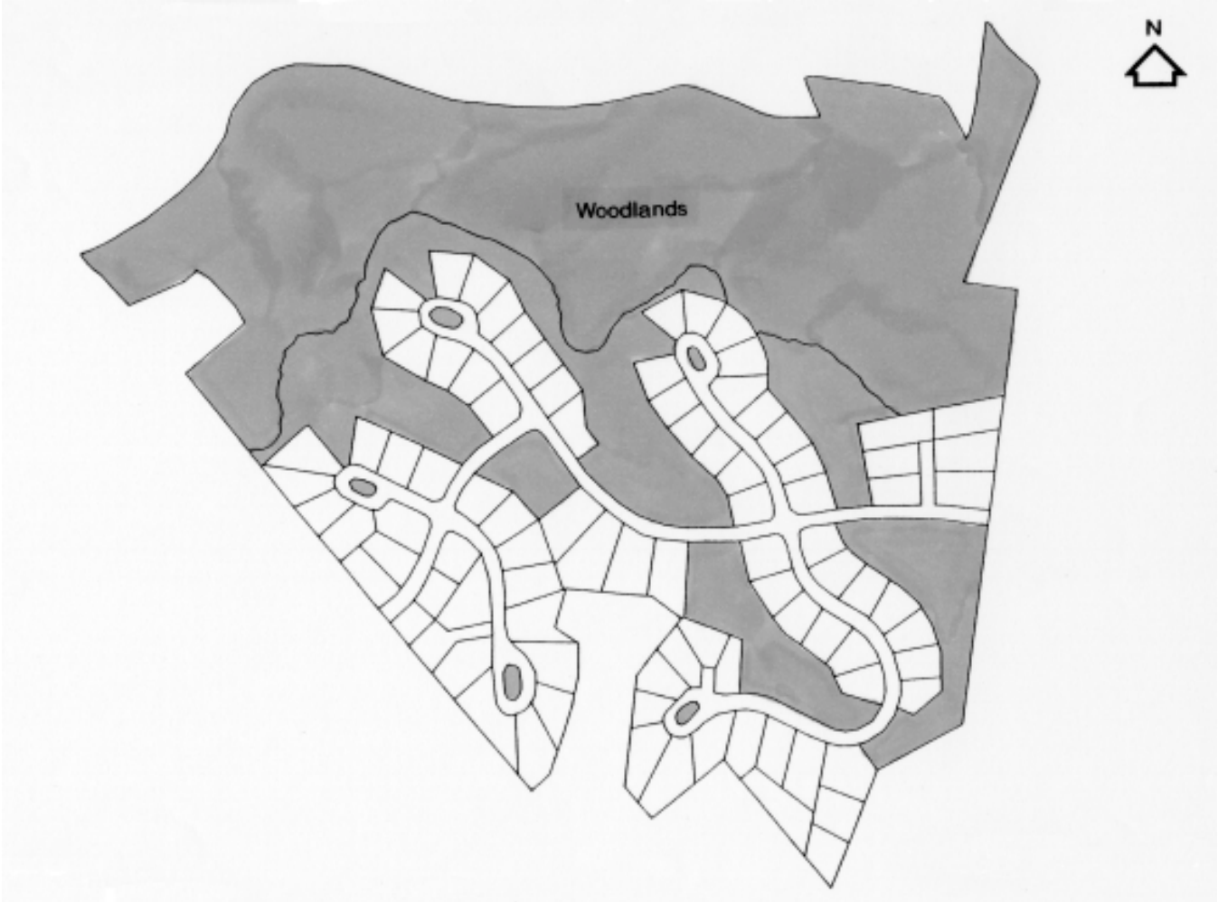
Figure 5-35 Natural Swale and Open Space Corridor Approach
