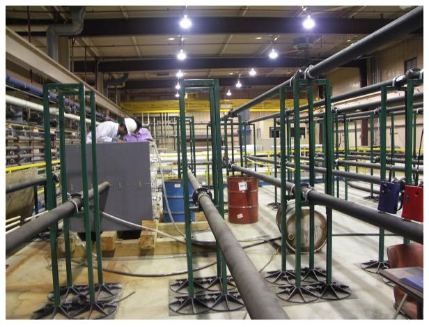
Current leak detection system being converted to hangar AFFF delivery system testbed
