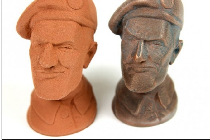
colorFabb (CF) filaments (Copperfill pictured, unpolished vs. polished)
