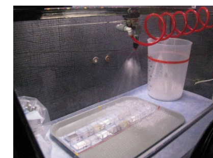
Spray application setup – EPA/Battelle
