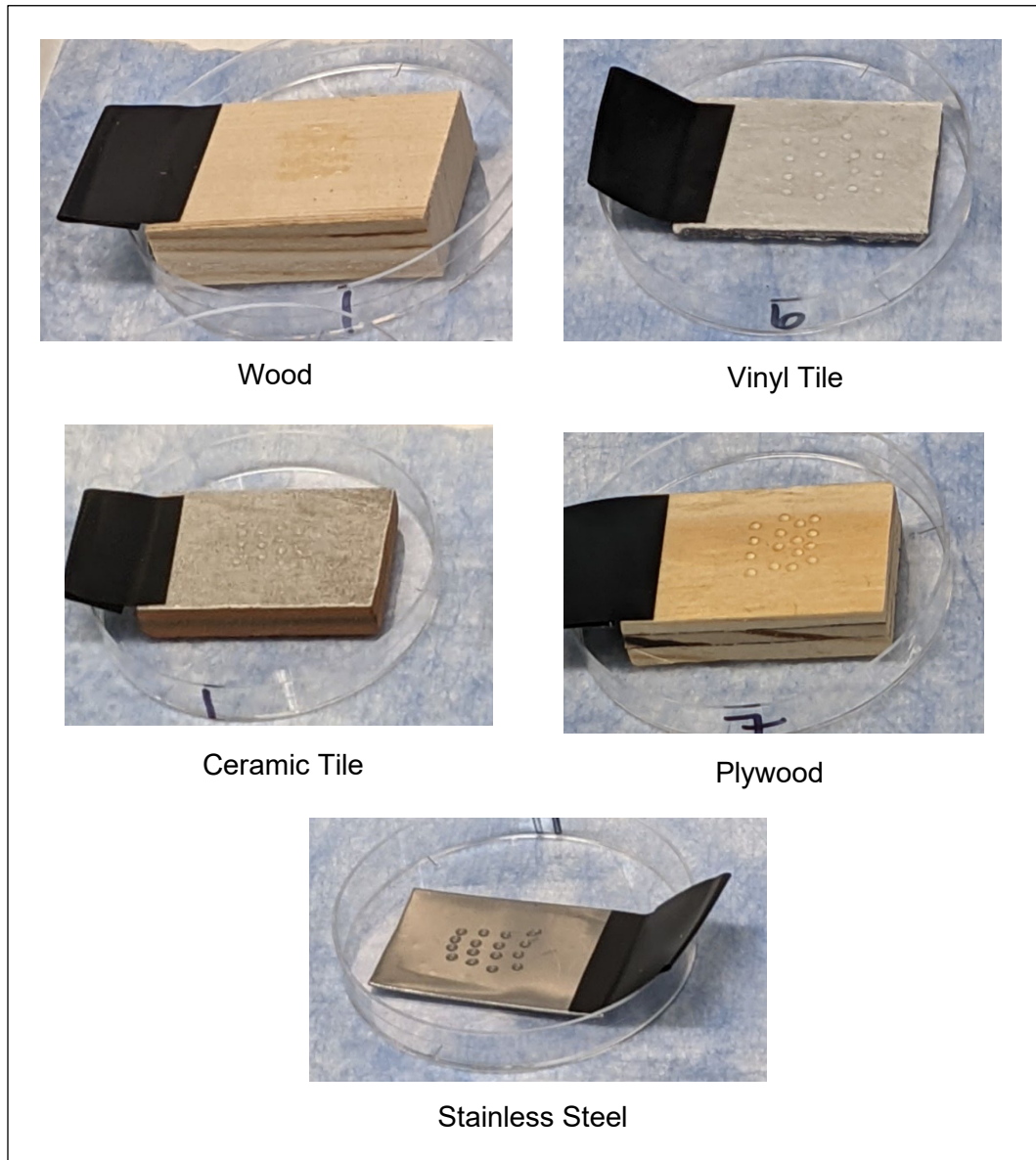
Figure 5. EA 6162 Solution Droplets Applied to Strippable Coating Coupons
