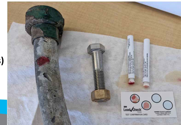
Surface swab kit turns pink for lead gooseneck but not for stainless steel
