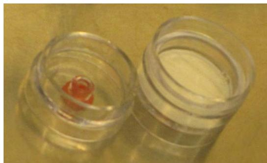
**Figure I-2. Vacuum Cassette with Top Section Removed**
