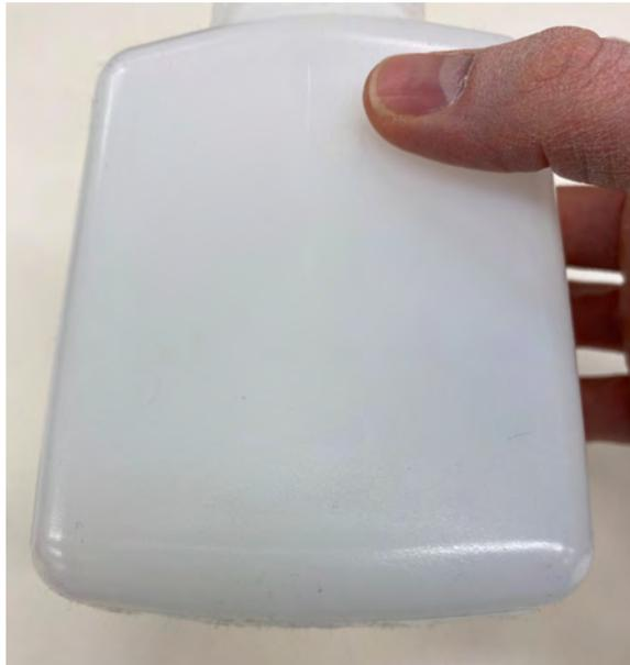
**Figure 62. Autoclaving HDPE Bottles Compromises their Structure**
