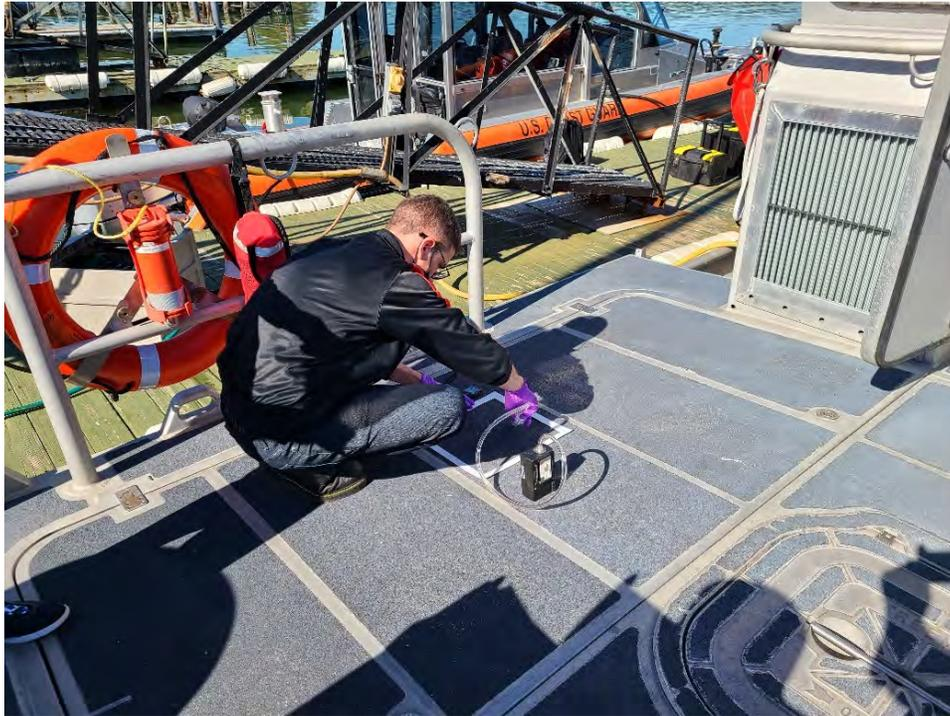
**Figure 19. Location of VFC Sampling of Nonskid Tread from the RBM.**
