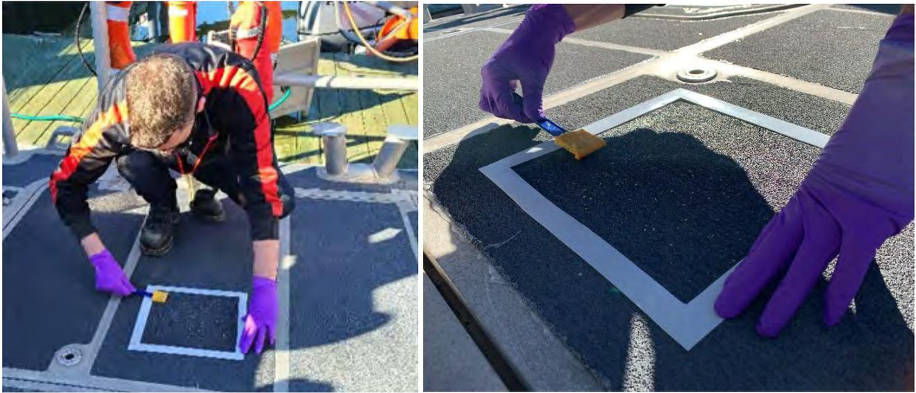
**Figure 15. Sponge Stick Sampling Location of Nonskid Tread from the RBS and RBM.**
