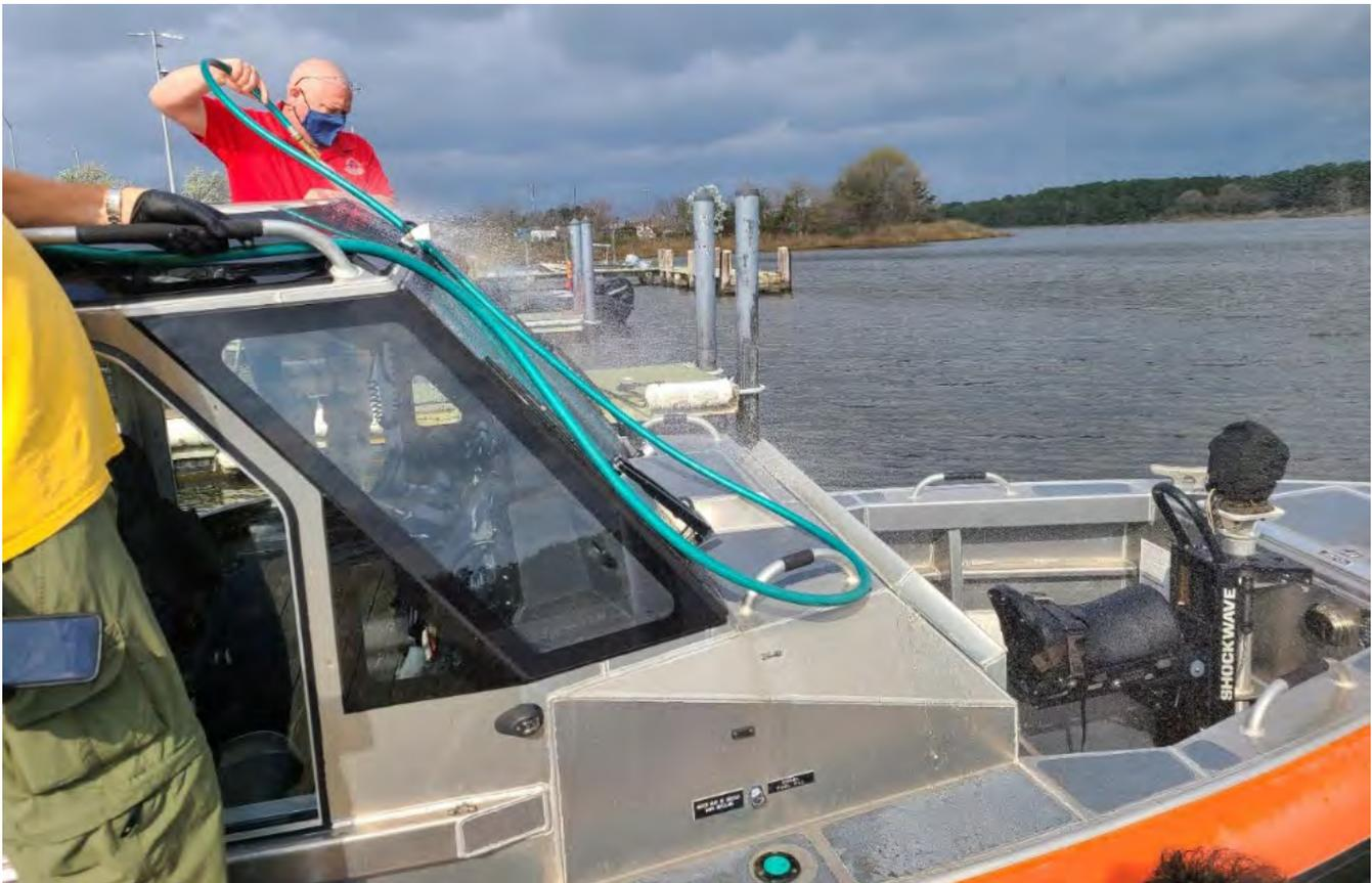
**Figure 23. RBS Washdown that Generated the Wash Water for Collection.**
