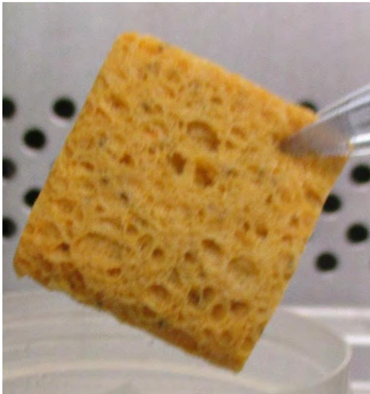
**Figure 14. Sponge Stick After Sampling Aluminum Surface of the RBS.**
