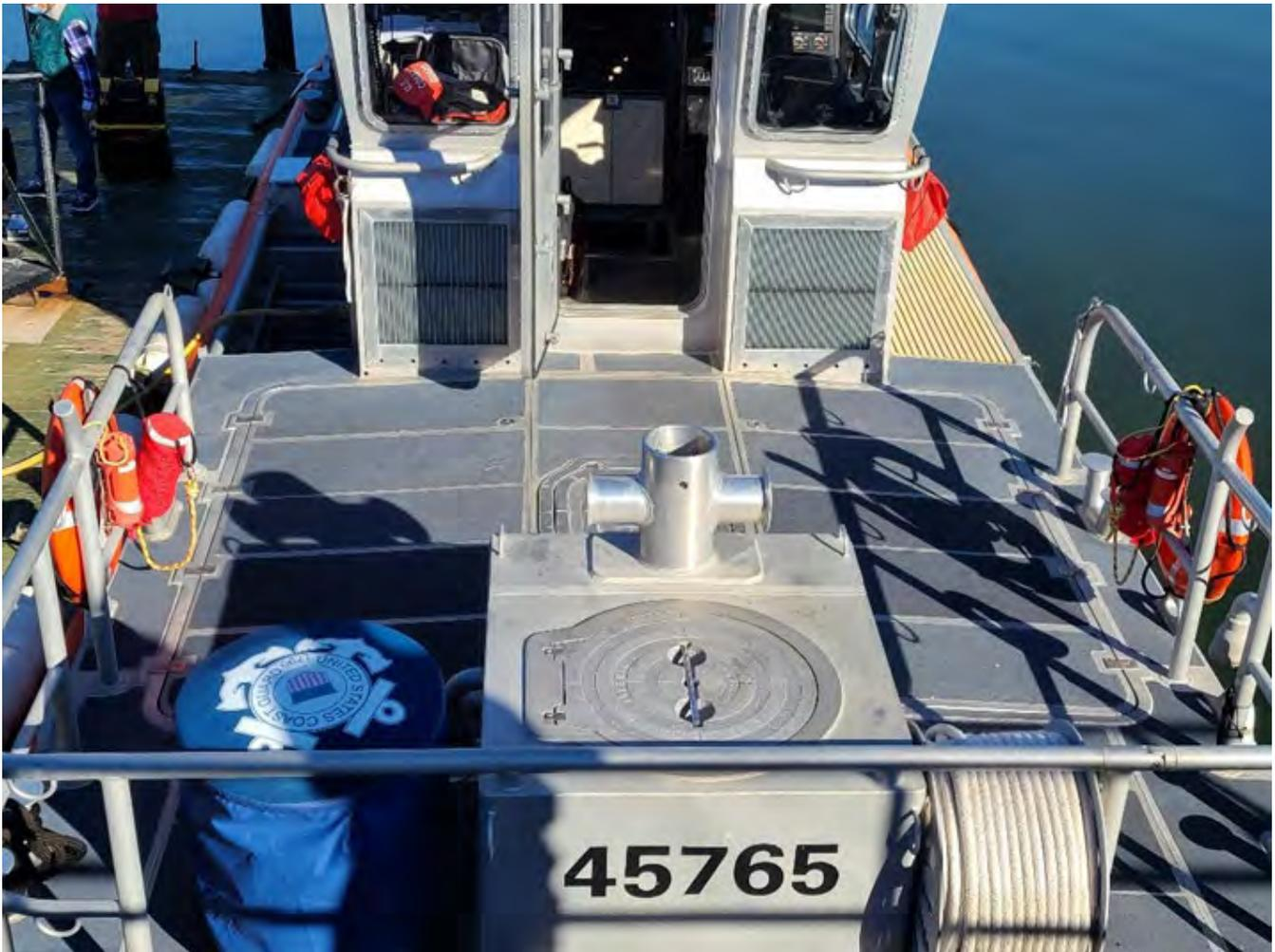
**Figure 5. Representative Deck Surface (Primarily Nonskid Tread with Some Aluminum) of an RBM Washed for the Collection of Wash Water Samples.**
