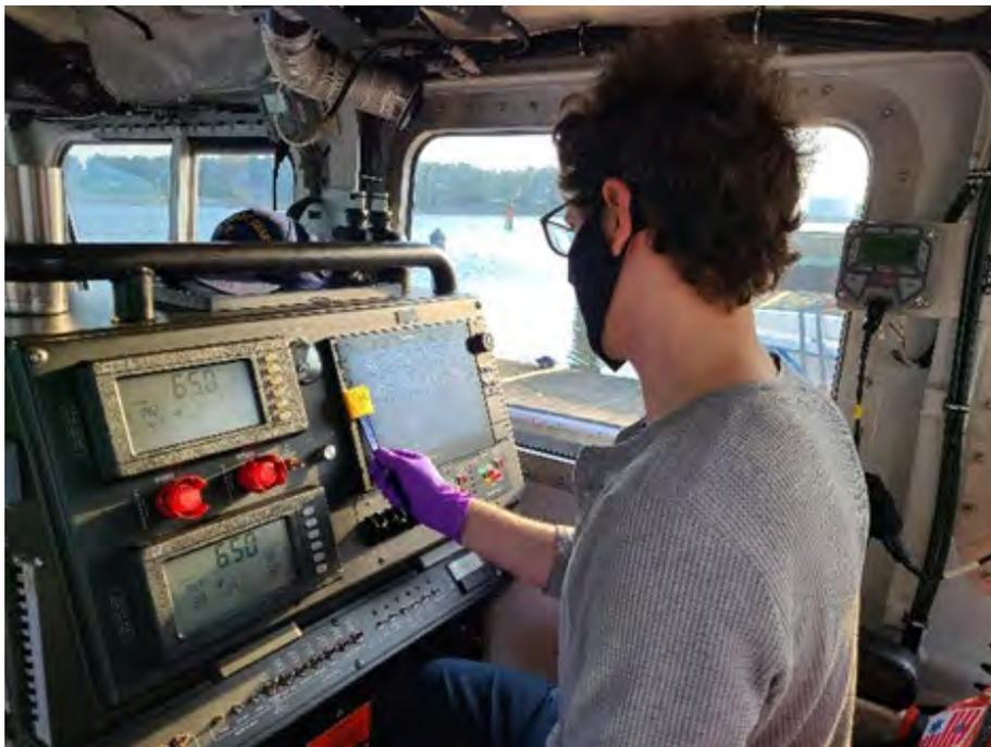
**Figure 17. Sponge Stick Sampling of On-Board Touchscreens from the RBM.**
