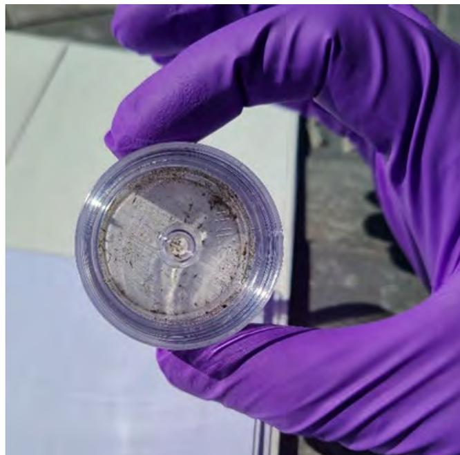
**Figure 20. VFC After Sampling Nonskid Tread Surface of the RBM.**
