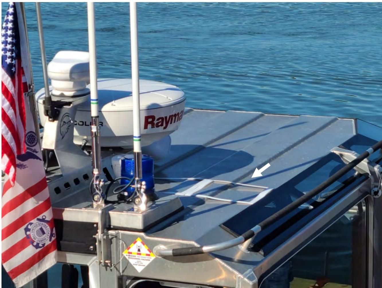
**Figure 1. Representative Area of Aluminum (Cabin Roof) Sampled on an RBS II (White Sampling Template Shown).**
