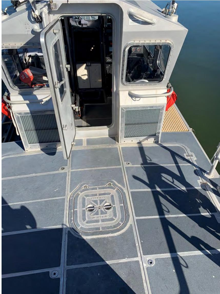
**Figure 2. Representative Nonskid Tread Adhered to Aluminum Surfaces Sampled on an RBM.**
