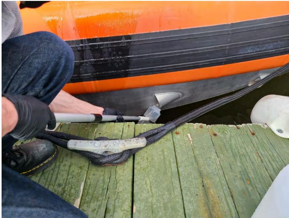
**Figure 24. Vessel Washdown Water Nontraditional Sampling Method Applied to an RBS Scupper.**
