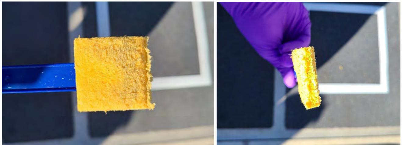
**Figure 16. Sponge Stick After Sampling Nonskid Tread from the RBS and RBM.**
