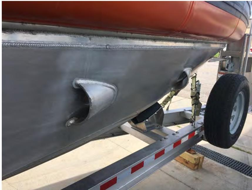
**Figure 11. RBS Starboard Stern Scupper.**
