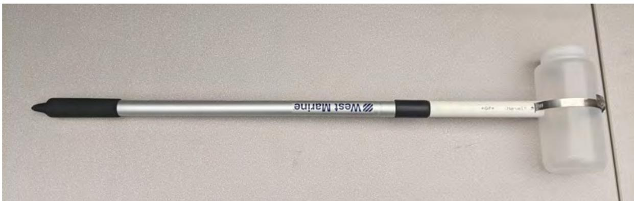
**Figure 12. Wash Water Runoff Collection Apparatus.**
