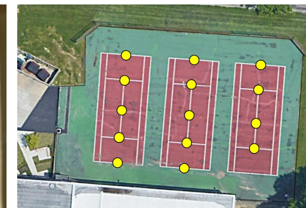
Fig. 7 Deployment map of the soda bottle rain gauges on the tennis courts near the DPHS rain garden.
