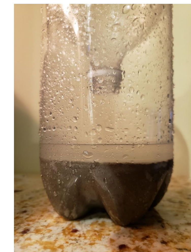
Fig. 6 Soda bottle rain gauge with collected rainfall. Gauges were constructed with 2L bottles, cement, and sealer.
