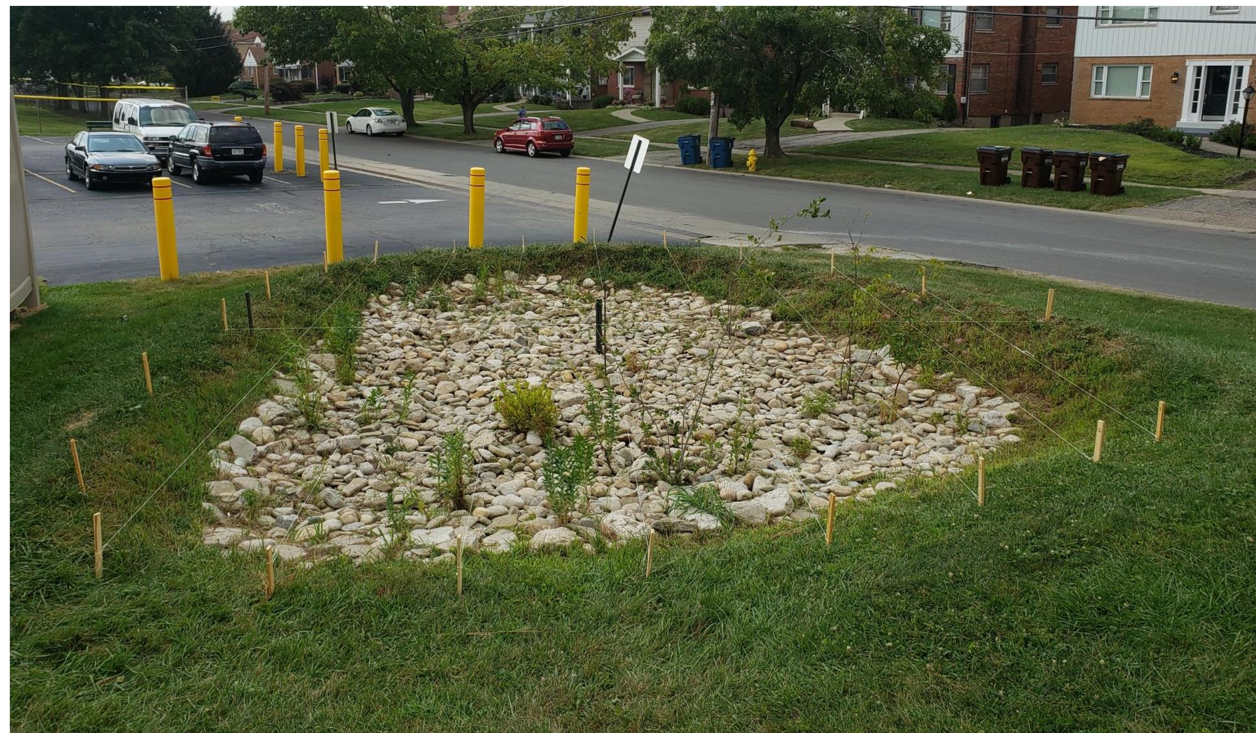
Fig. 1 The Deer Park High School rain garden. Stakes were placed around the perimeter and across the rain garden to create 8 transects. White string was attached to the transect stakes so the string remained at a common elevation from which students could measure.
