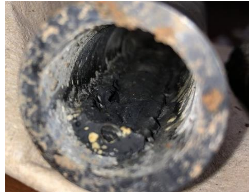
Service line with melted plastic pooled inside.
