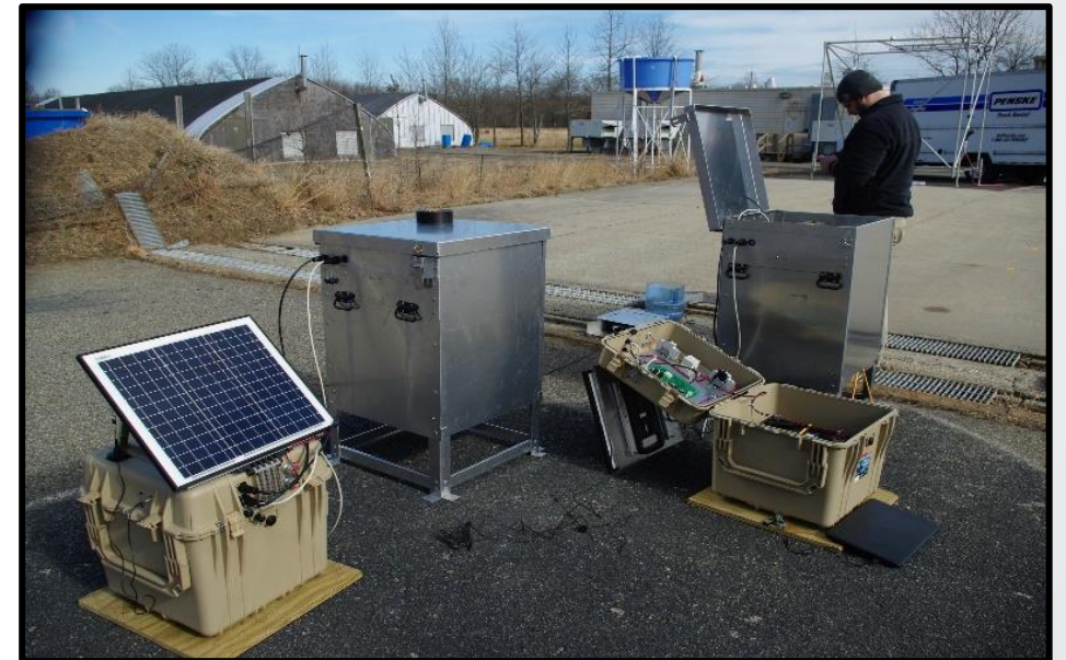
Autosamplers with cell phone activated sample triggering
