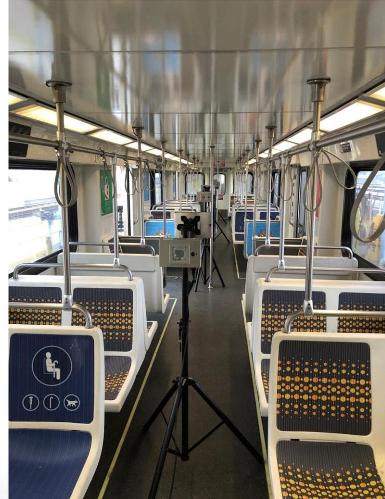
\* Dose as measured with LA light sensor (ILT SED270) in metro car (which includes UVC + UVB + UVA)
