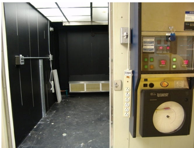
Figure 3-2. T- and RH-Controlled Environmental Storage Chamber
