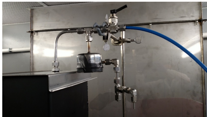
Figure 3-5. Micro-Venturi Eductor Fitted with Large Particle Separator
