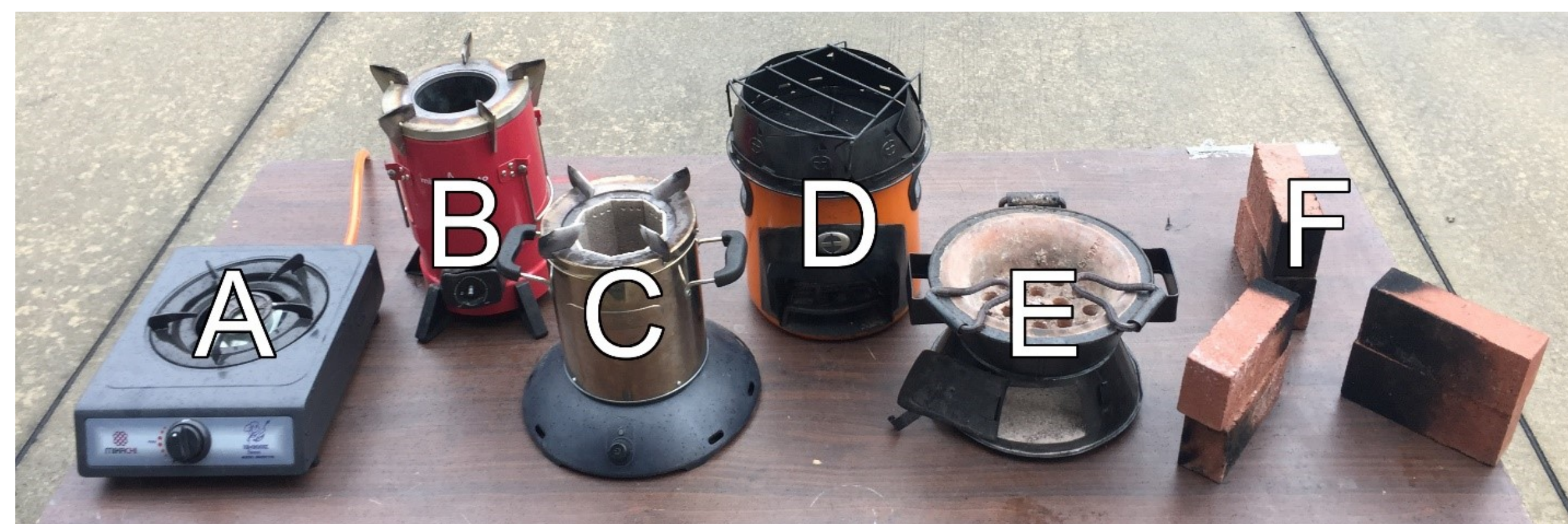
Figure 1. Photo of the six stove types tested: (A) LPG – Mikachi, (B) Pellet – Mimi Moto, (C) Wood Fan – Philips HD4012, (D) Wood Rocket – Envirofit G3300, (E) Charcoal – Kenya Ceramic Jiko, and (F) Wood Traditional – Three Stone Fire
