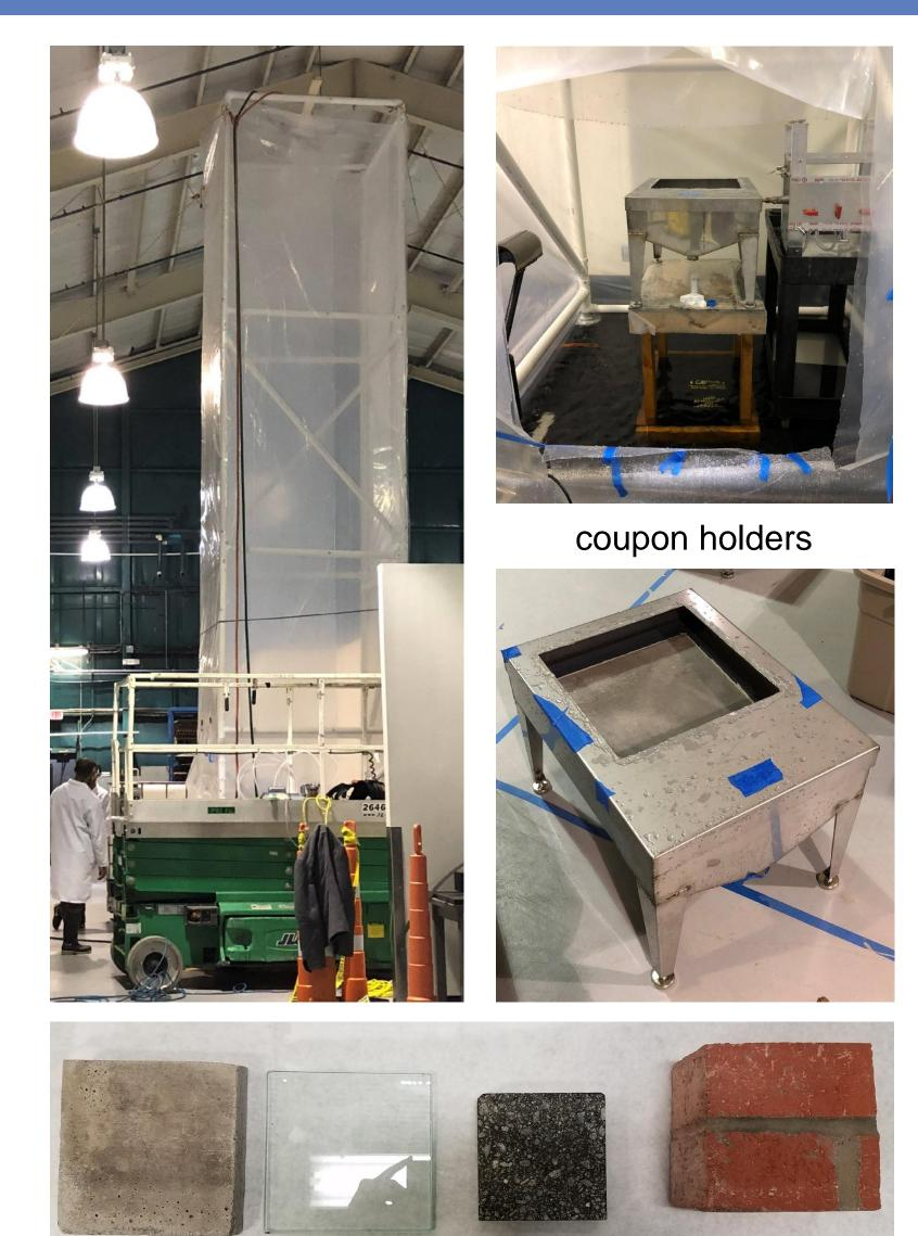
types of materials tested: concrete, glass, asphalt, brick
