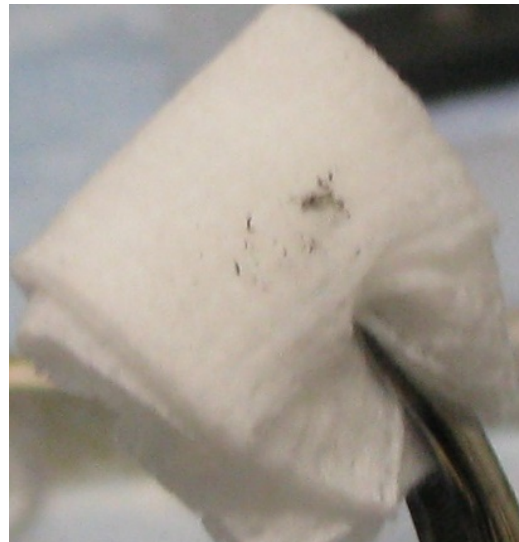
Figure 13. ABS plastic debris on wipe sample.
