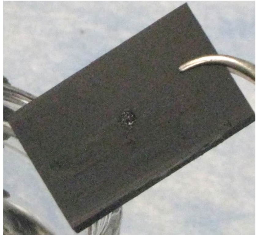
Figure 11. Damage to ABS plastic caused by HD (3).
