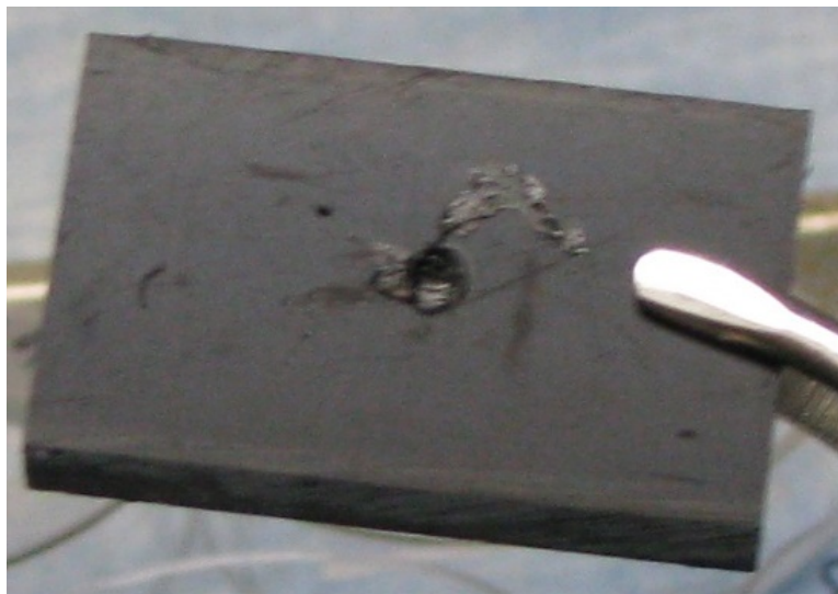
Figure 12. Damage to ABS plastic caused by HD (4).
