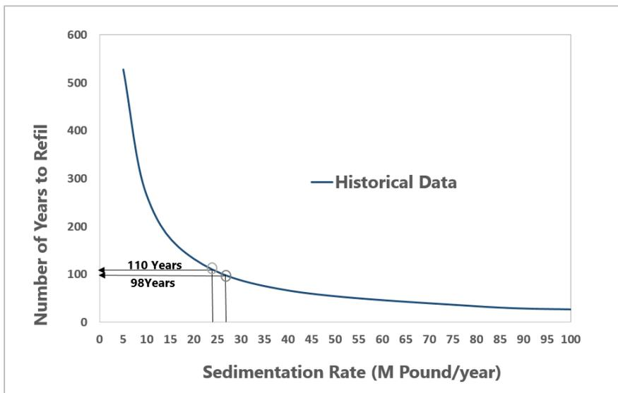
Figure 16 [B]. Refill time as a function of sedimentation rate in units of million ibs/year. Based on the historic sediment accumulation rate of 24 million ibs/year, it
