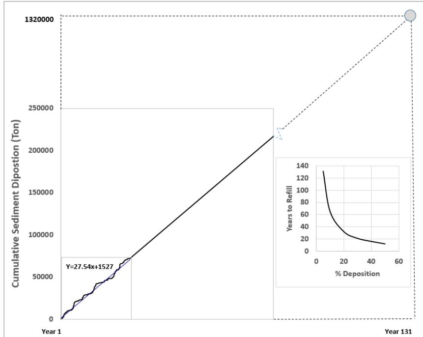
Figure 16 [A]. SWAT computed and regressed cumulative sediment accumulation vs. time in years. The lower left corner is SWAT computed values for the period 2010-2016. The inset panel shows refill time as a function of percentage sediment loading retained.
