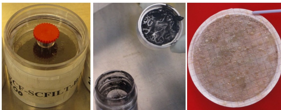
Figure 47. Subway Car Filter (SCFILT) Representative Images, Sample Receipt, Addition of Extraction Buffer, and Culture Growth on SBA Filter Spiked with 30, 300, or 3,000 Spores (from left to right, respectively)
