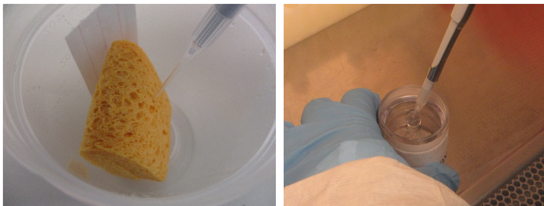
Figure 5. Sponge-Stick (left) and Vacuum Filter Cassette (right) After Spiking with the B. a. Sterne Suspension
