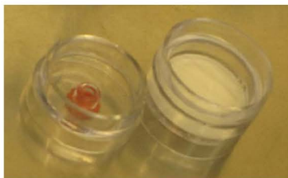
Figure 1. Vacuum Cassette with Top Section Removed
