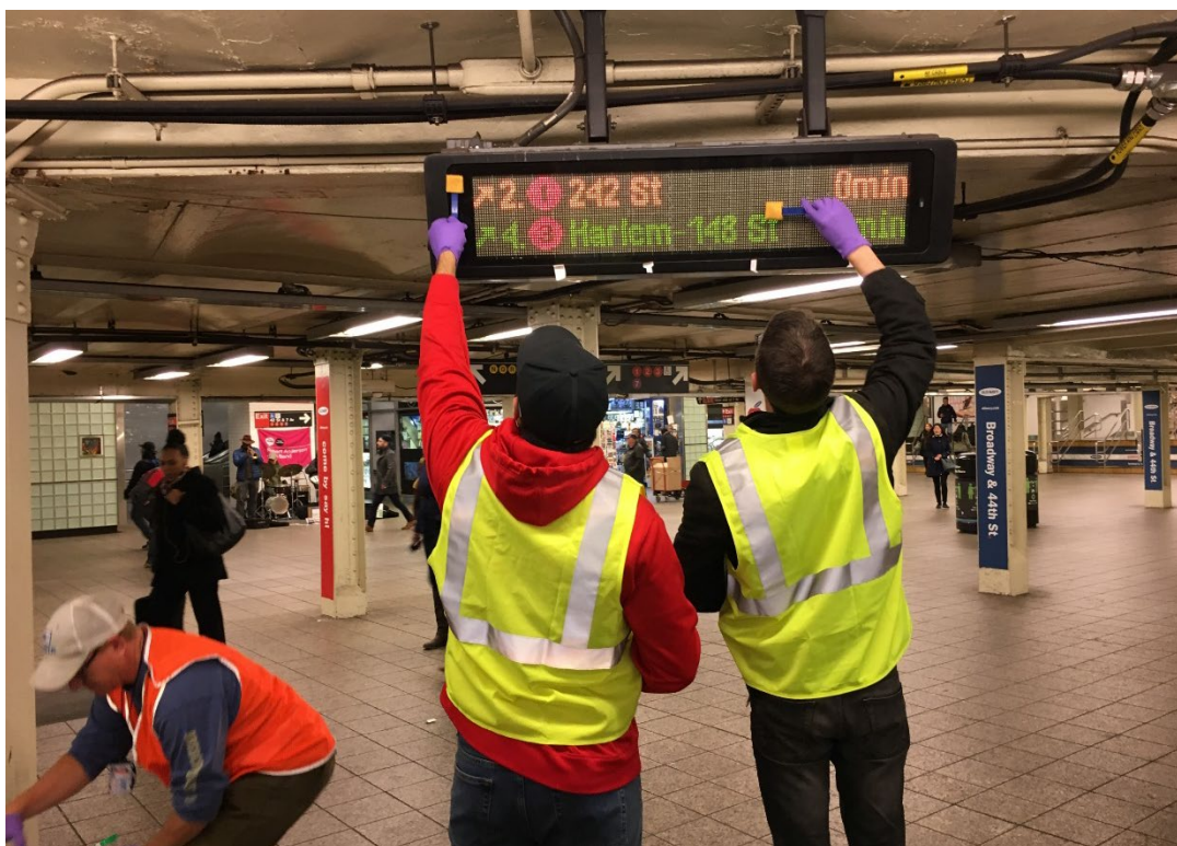
Figure A-4. Electronic Display Panels (Below Ground) Located in Times Square 42 nd Street Station, Near Track 3 – Sampled with Sponge-Sticks
