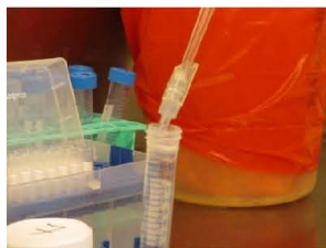
Figure 3. Nozzle Removal Using 1 mL Pipette
