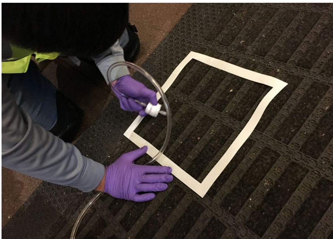
Figure A-1. Carpet Surface Located by the Jackie O Entrance to Station, Off 42 nd Street – Sampled with Vacuum Filter Cassette
