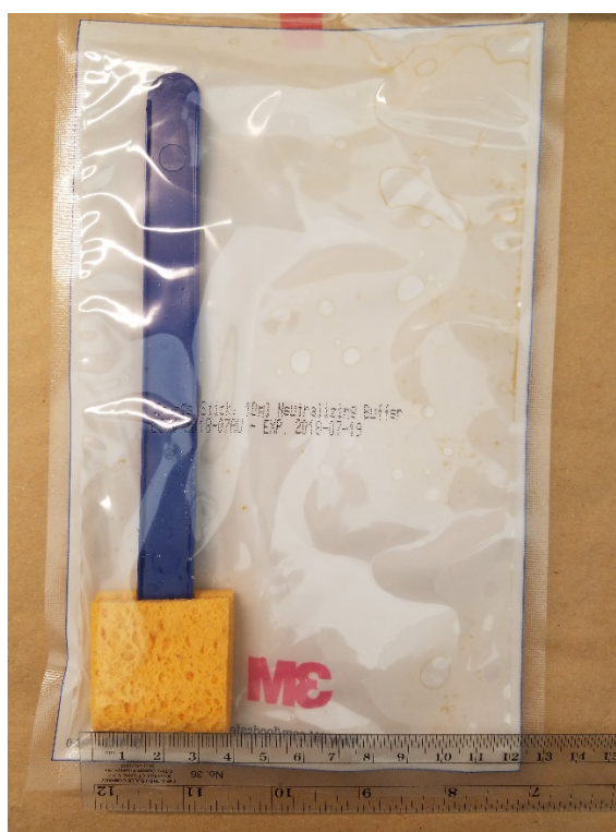
Figure 1. Pre-Wetted Sponge-Stick from 3M Used for Surface Sampling
