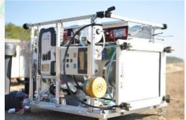
The EPA “Flyer”: An unmanned, telemetry-controlled sampling system
