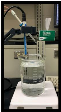
Image 1 – Photograph of titration apparatus used in experiments
