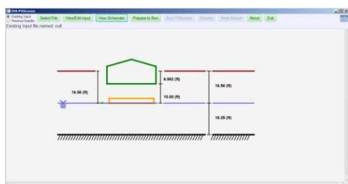
Figure 2. PVIScreen schematic of petroleum vapor intrusion scenario.
