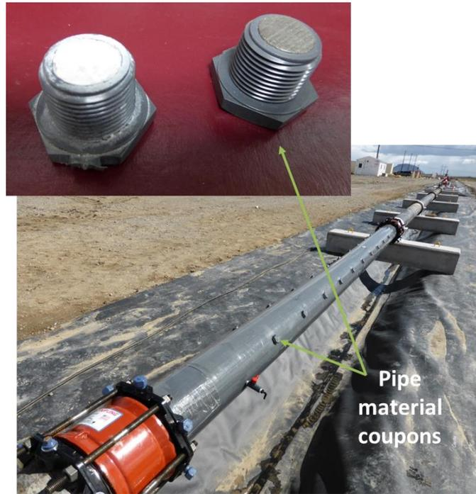
**Figure 3: Coupons used to sample the interior pipe surface.**
