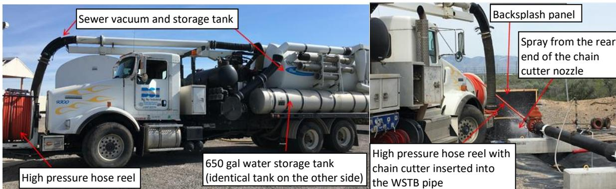
**Figure 5: A combination truck (left), and a nozzle being inserted into the Water Security Test Bed pipe for decontamination (right).**
