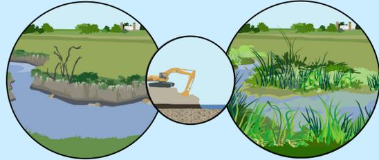
**Figure 1. Big Spring Run Restoration Event.** Restoration to remove legacy sediments was conducted at Big Spring Run beginning in October 2011, and ending November 2011. Mill pond reservoir sediment stacks, i.e. 'legacy sediment', were cleared away, exposing the once-buried relic hydric soil (Holocene *pre-settlement* wetlands on Pleistocene gravel), leading to drops in base level and the widening of channels (Walter & Merritts 2008).
