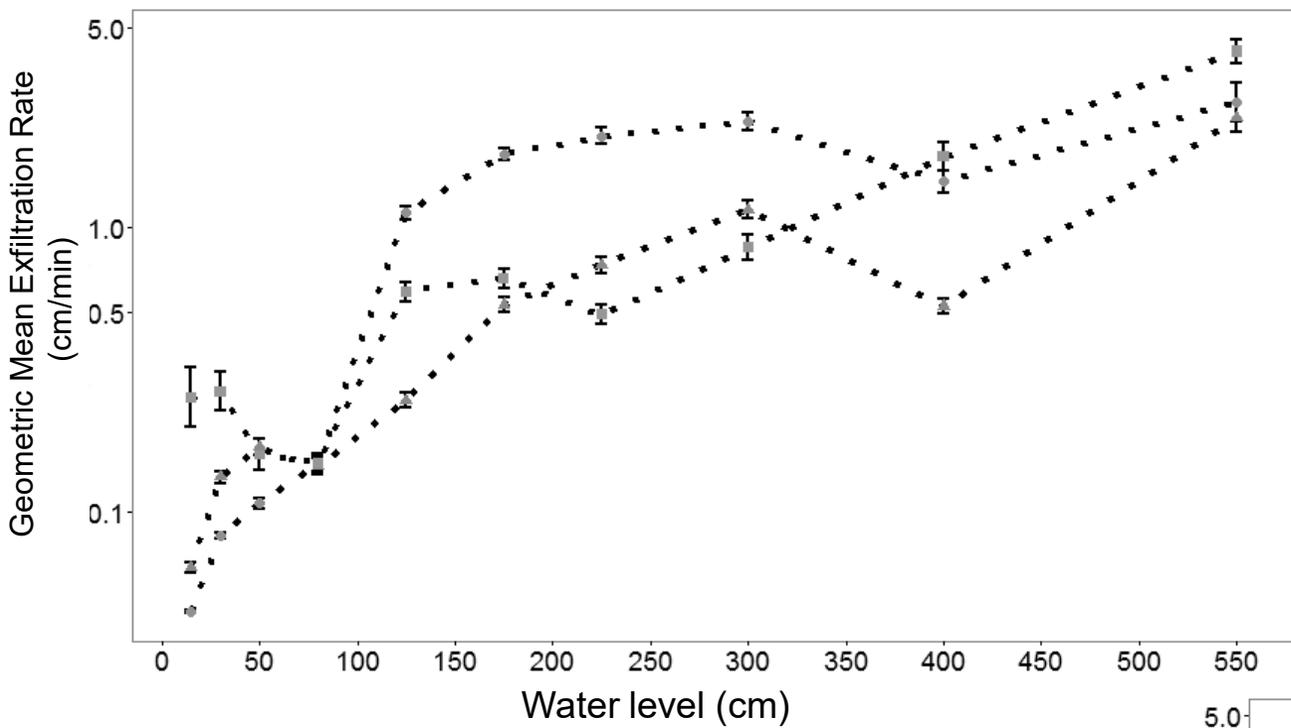
The expected edge effect was noted for strip 10D when the water level was larger than 100 cm.
