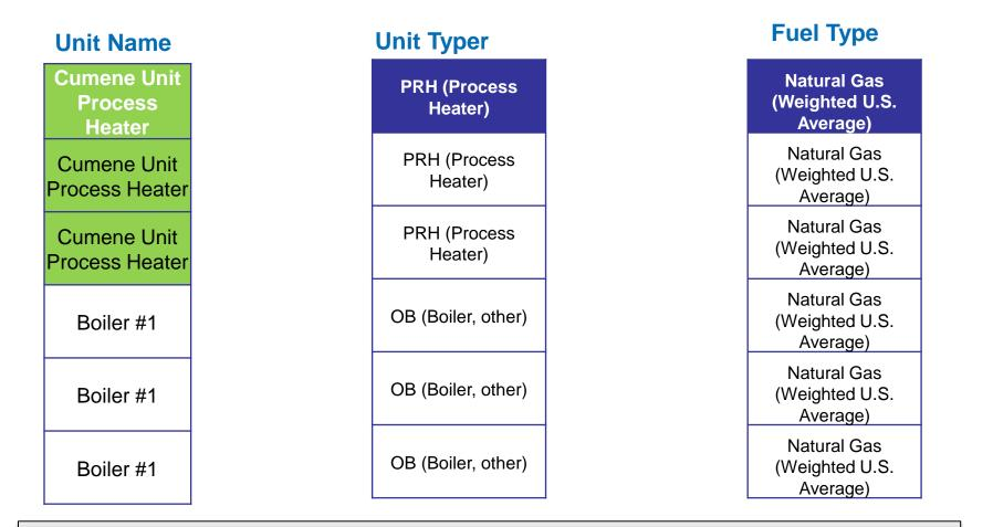
Map combined unit type/fuel type/capacity to NEI's Source Classification Codes
