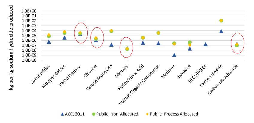
22 Air Emissions Completely Filtered from Sodium Hydroxide Inventory with Process Allocation
