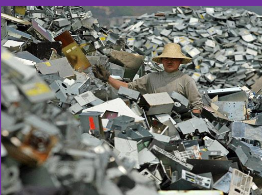
Migrant workers cracking piles of burned computer components to remove the copper in the burn village, Guiyu, China, May 2008. ©2008 Basel Action Network (BAN)
