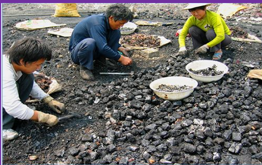
Migrant workers cracking piles of burned computer components to remove the copper in the burn village, Guiyu, China, May 2008. ©2008 Basel Action Network (BAN)
