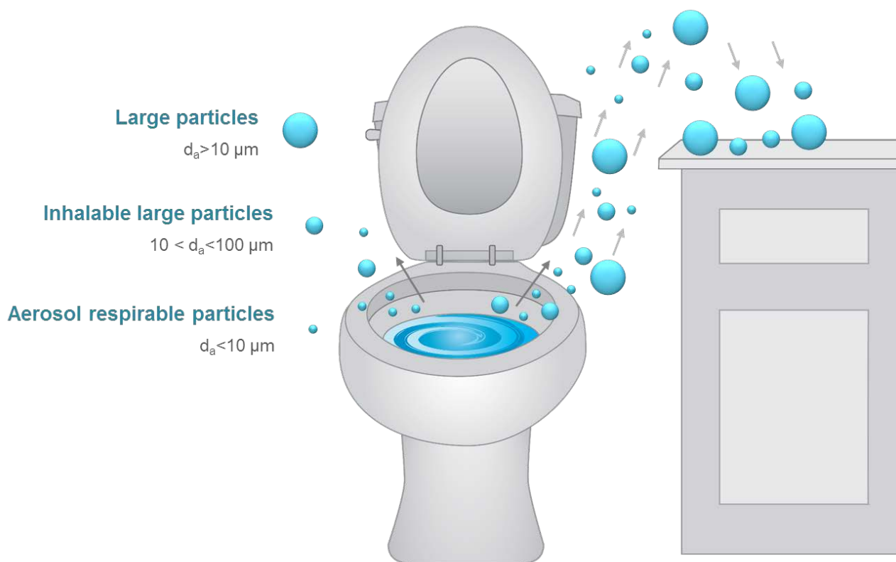
Figure 4-2. Toilet flush showing aerosol and particle deposition.
