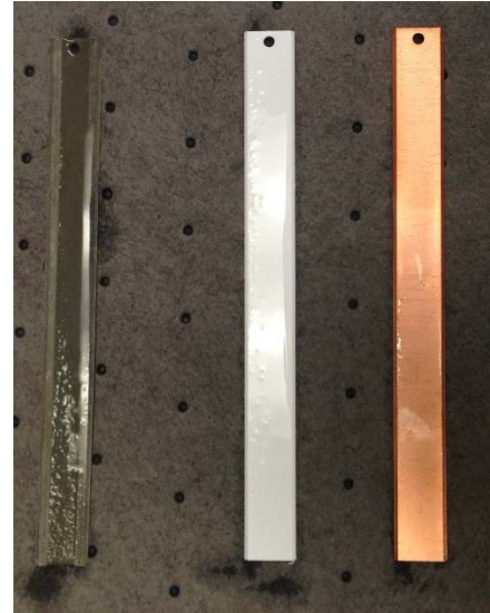
Figure 9. Testing coupons with biofilm growth: concrete-lined (left), PVC (middle), and copper (right).
