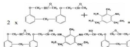
Figure 3. Two molecules of EPON 862 bonded with one molecule of curing agent W into a unit cell
