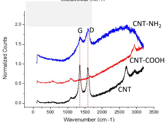
The Raman band of the functionalized NTs shifted to higher wavenumber → intertube interaction is less and physical interaction of the polymer
