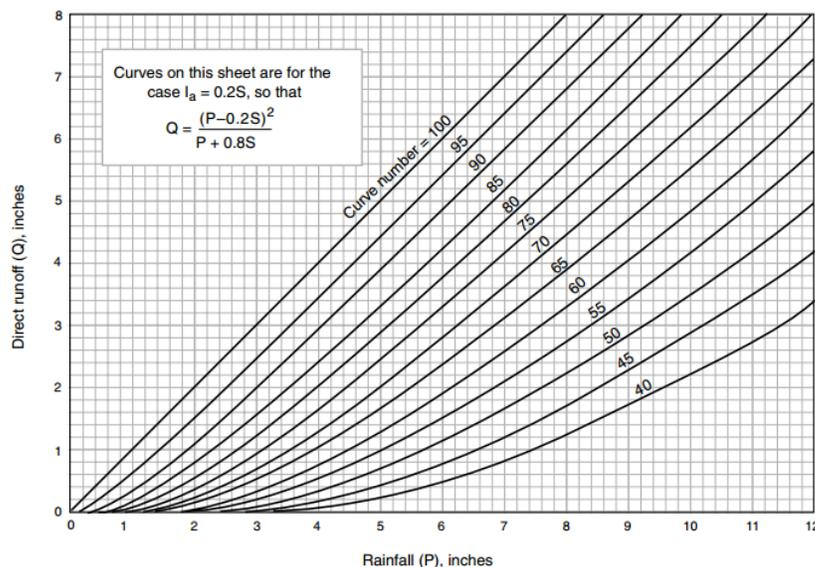
Figure 3. A visualization of the empirical Curve Number method shows the relationship between rainfall inputs and runoff outputs where  $I_a$  is initial abstraction,  $S$  is the retention parameter,  $P$  is precipitation, and  $Q$  is runoff. Image from (USDA, 1986)
