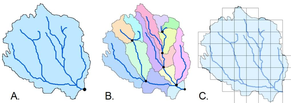
Figure 6. Visualization of the spatial structure in runoff models. A: Lumped model, B: Semi-Distributed model by sub-catchment, C: Distributed model by grid cell. Runoff is calculated for each sub-catchment at the pour point represented by the black dots in Fig. 6B. Distributed models calculate runoff for each grid cell, while lumped
