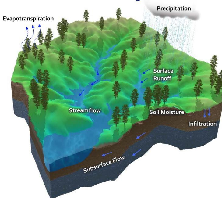
Figure 1. A simplified diagram of the hydrological cycle governed by the water balance equation (Brewster, 2017; ESRI, 2015).
