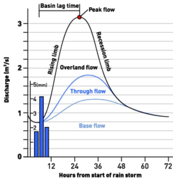
Figure 7. Shows a hydrograph of observed discharge data separated into model components of Baseflow, Throughflow, and Overland flow.
