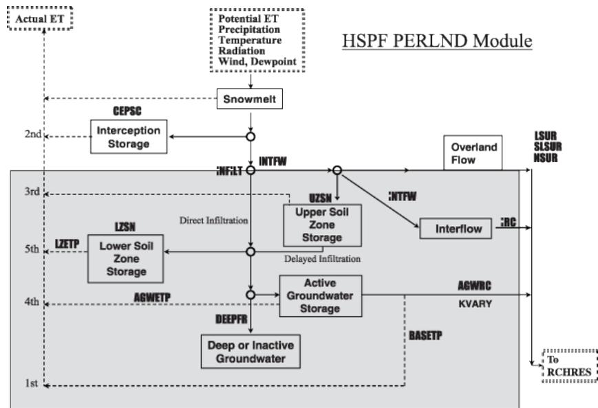
Figure 4. The conceptual model HSPF schematic shows the Pervious Land segment module (PERLND) as an assembly of multiple storage processes following the water balance equation. Image from (Atkins et al., 2005)
