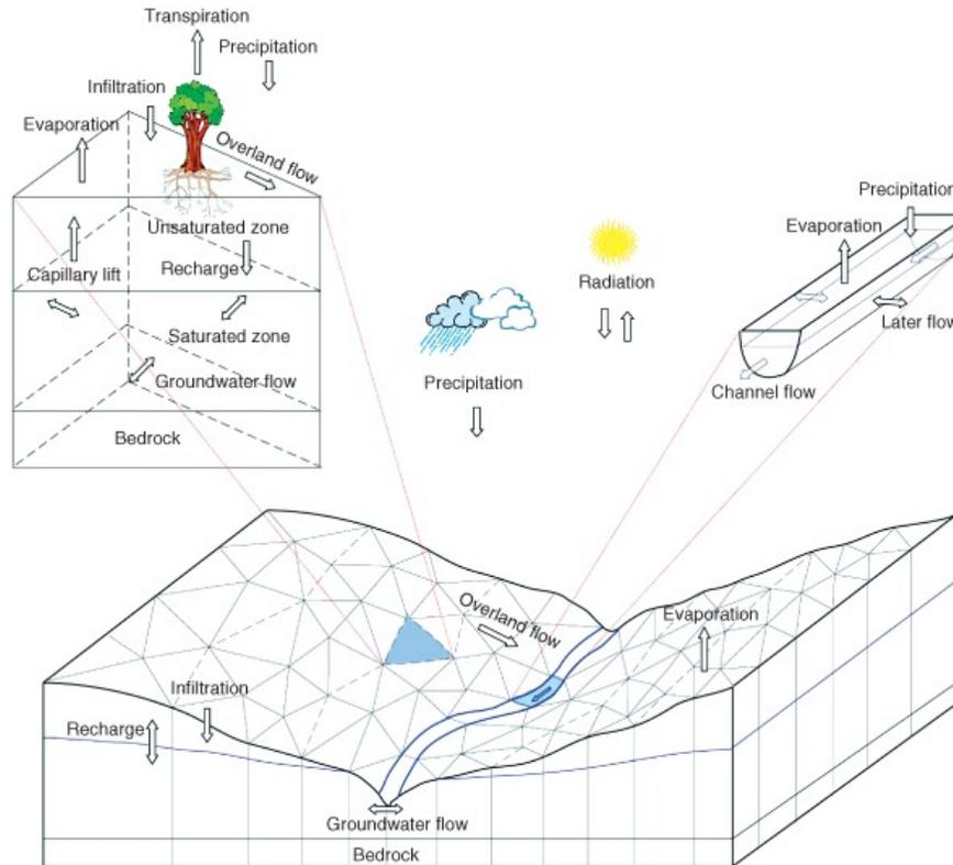
Figure 5. The model structure of the physically-based Penn State Integrated Hydrologic Modeling System (PIHM). It shows physical movement of water through each Triangular Irregular Network via overland flow, evapotranspiration, infiltration, recharge, and groundwater. Image from Qu (2004).
