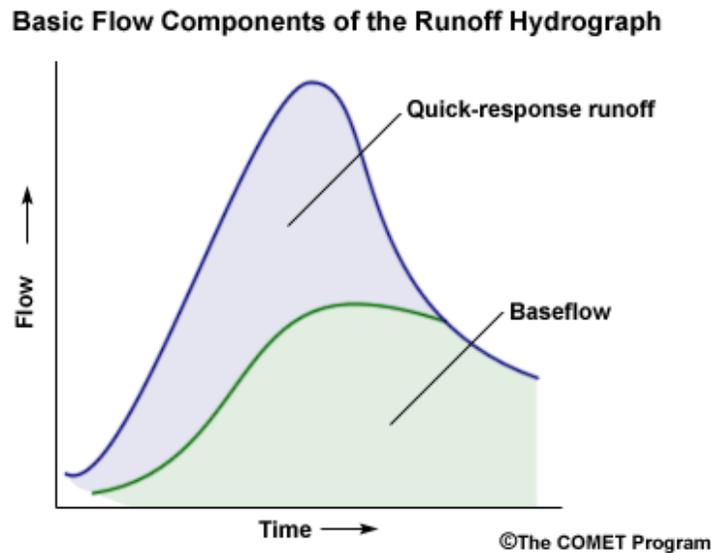
Figure 2. The unit hydrograph separation into quick response runoff from a storm event and baseflow. Image from (UCAR., 2010)
