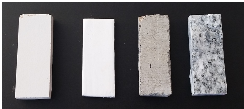
Figure 2-1. Coupons not covered with simulated subway grime. From left to right: ceramic tile, painted carbon steel, weathered concrete, and granite.
