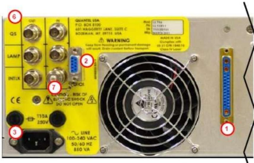
Figure E-1. Back side of LII 300 unit (top photo) and laser power supply (two bottom photos) with marked connections.
