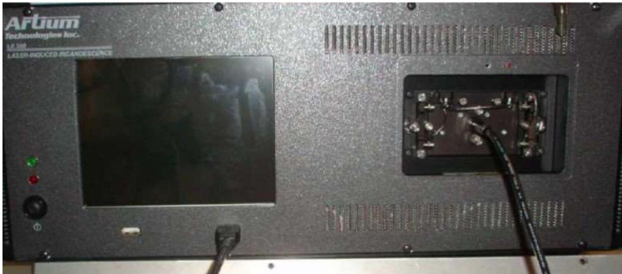
**Figure E-7. Front panel of the LII 300 unit showing the operational check lamp.**
