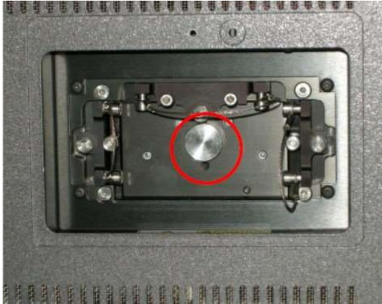
**Figure E-6. Front panel of the LII 300 showing the sample cell access door.**
