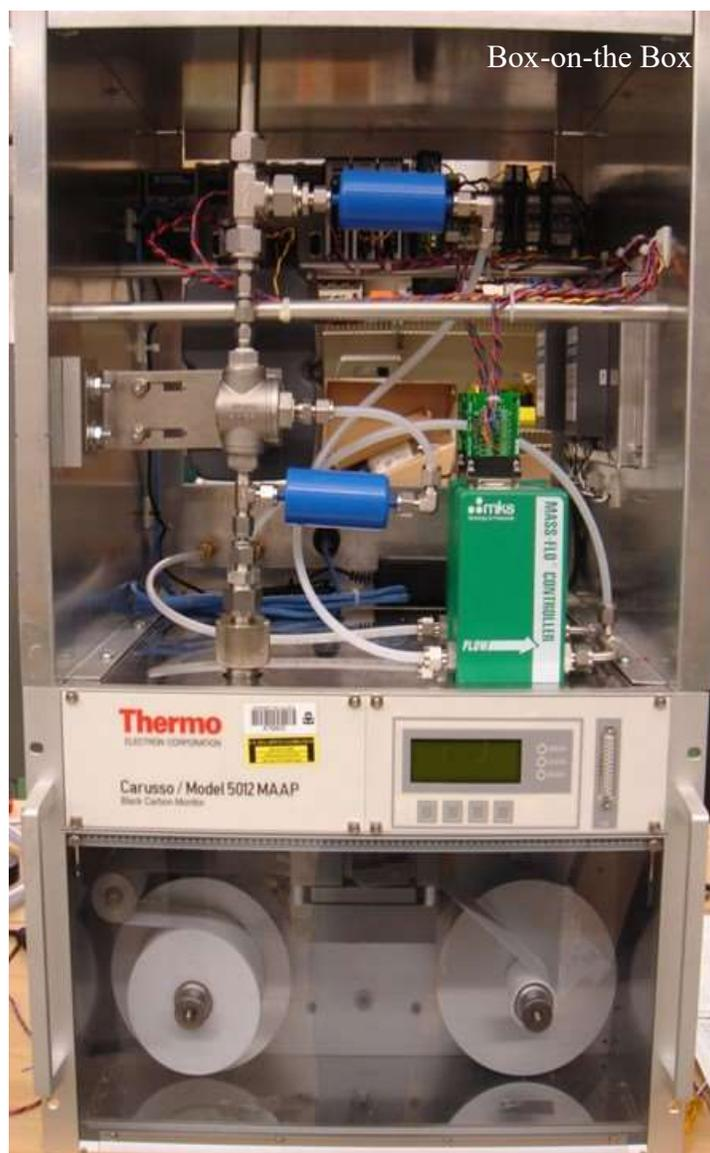
Figure D-1. Modified MAAP Model 5012 showing the “box-on-the-box.”
