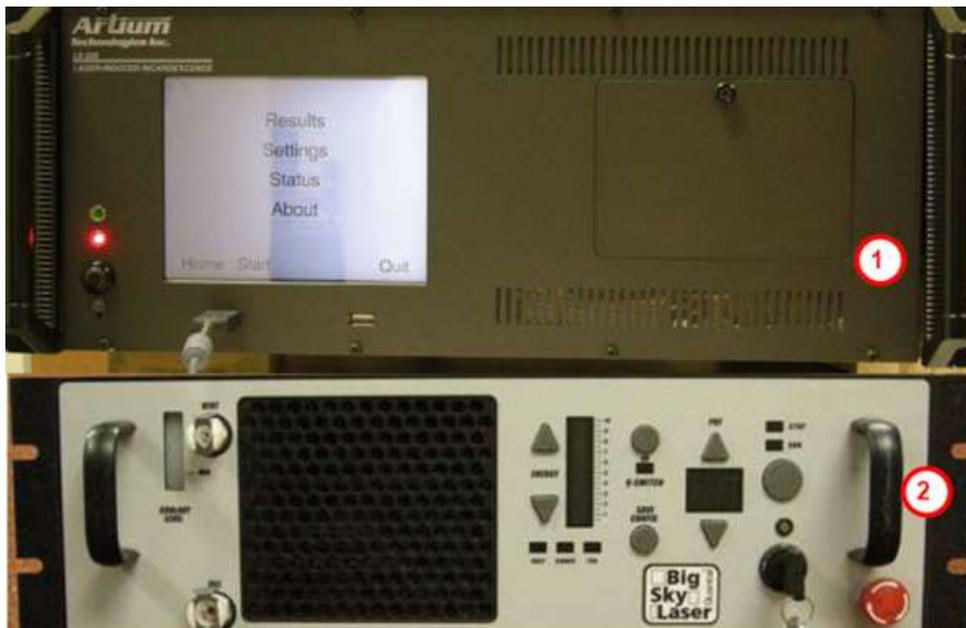
**Figure 3-12. Major components of the LII 300: (1) self-contained LII 300 instrument and (2) laser power supply.**
