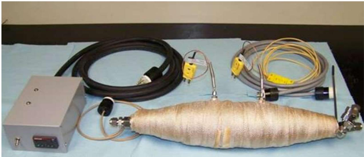
**Figure 3-5. Components of the catalytic stripper system.**
