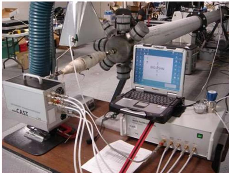
Figure 3-4. MiniCAST, primary diluter, and catalytic stripper installed on the flow tunnel.
