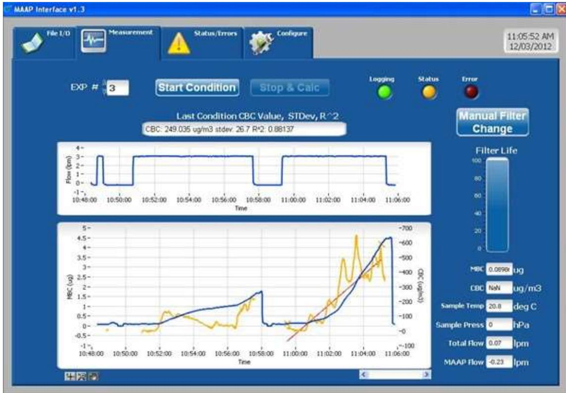
Figure C-11. Updated SuperMAAP measurement screen (note yellow status light is on).
