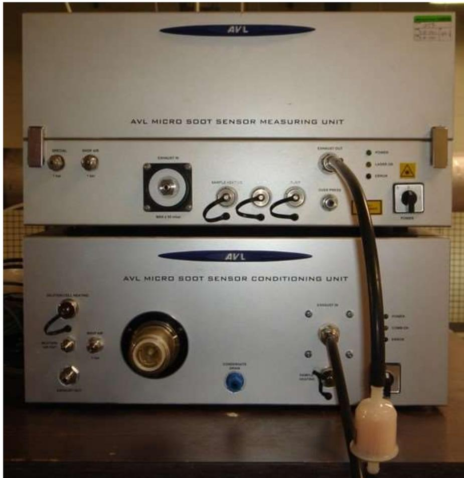
**Figure F-2. Connections between measuring device and conditioning unit – front side.**
