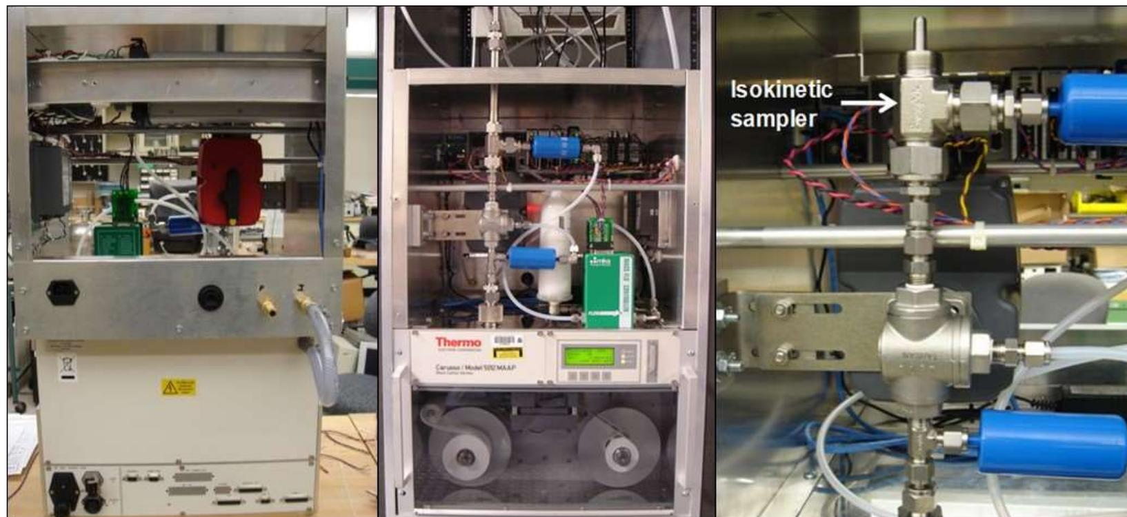
**Figure C-4. Front and back views of the SuperMAAP showing original hardware configuration based on workshop discussions.**
