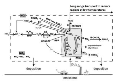
Figure 2-1, Schematic diagram of the cycle of reactive, oxidized nitrogen species in the atmosphere Source: National Center for Environmental Assessment.
