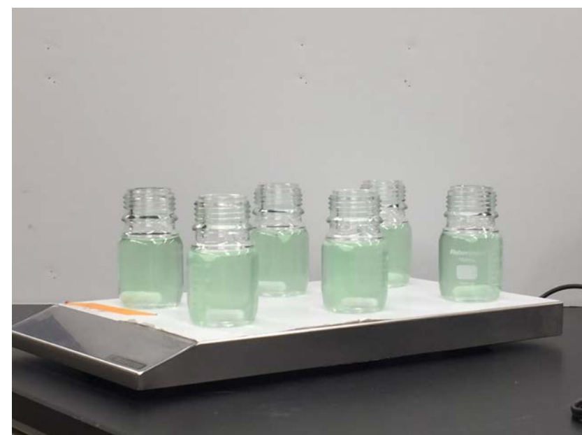
Jar Test set up including duplicate control, 30 minute suspension and 24 hour suspension jars.
