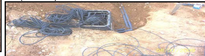
Water content reflectometer (WCR) installation
