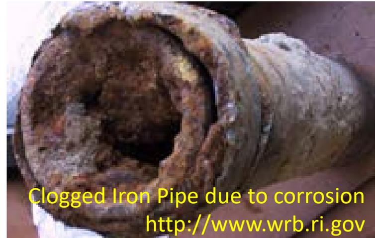
Clogged Iron Pipe due to corrosion
