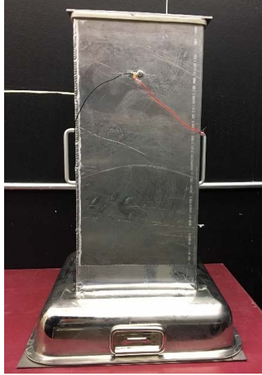
Figure 3-6. Spray-Dry Deposition Stack Modified for Ballast Coupon Deposition
