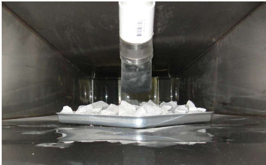
Figure 3-4. Leaf Blower Nozzle and Ballast Coupon Inside AA Sampling Wind Tunnel
