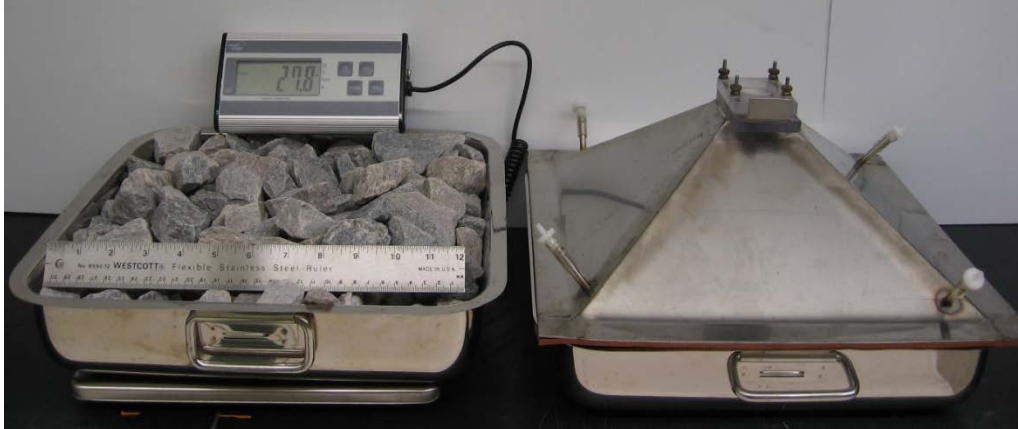
Figure 2-10. Ballast Coupons Showing Size and Weight in Pounds (left) and ADA Attachment (right)
