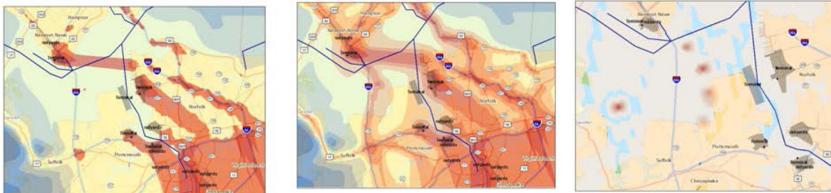
Figure 7: C-PORT Benzene concentration differences after expanded port scenario
