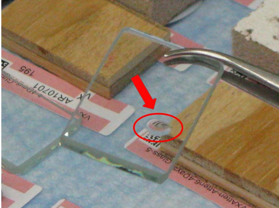
**Figure 3. Photograph of silanized glass coupon with VX having a “pancake” appearance.**
