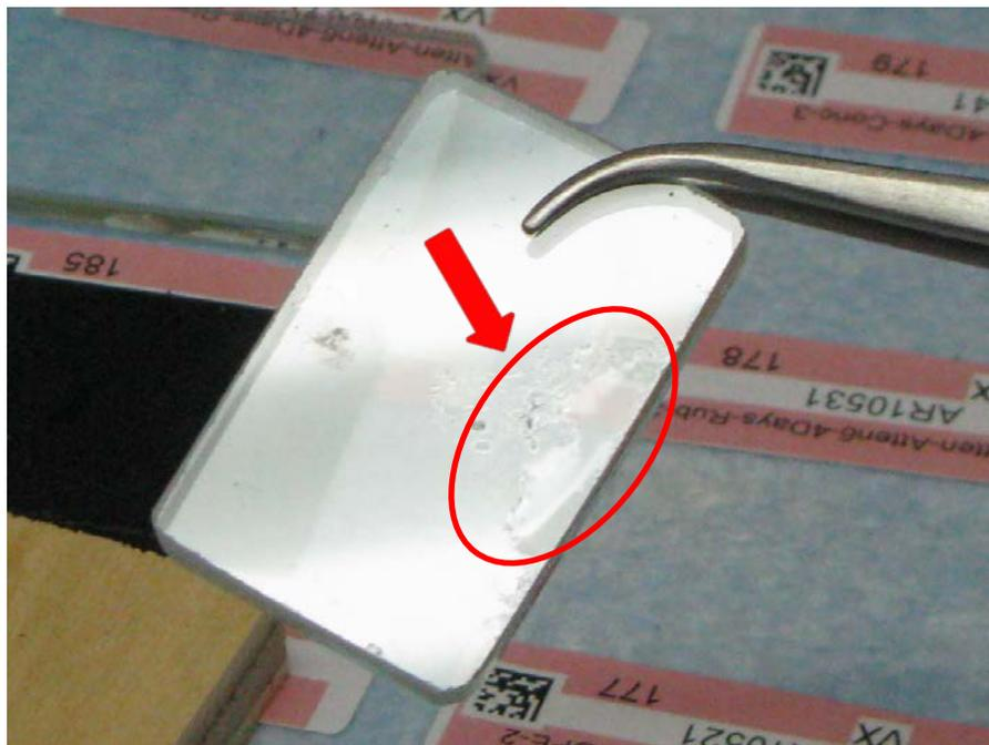
**Figure 4. Photograph of silanized glass coupon with VX having a “spread” appearance.**
