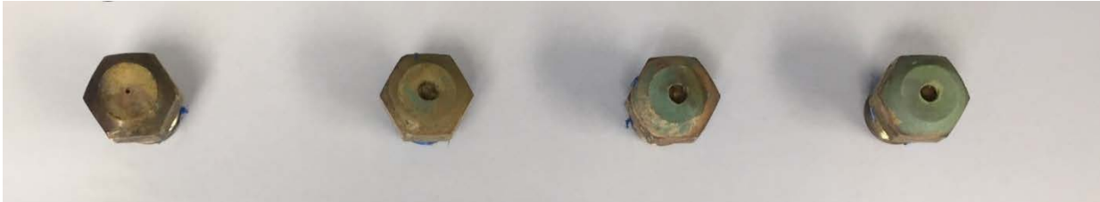
Figure 7-2. Dust Boss nozzle failure. From left: control, test 1 test 2 and test 3 nozzles.
