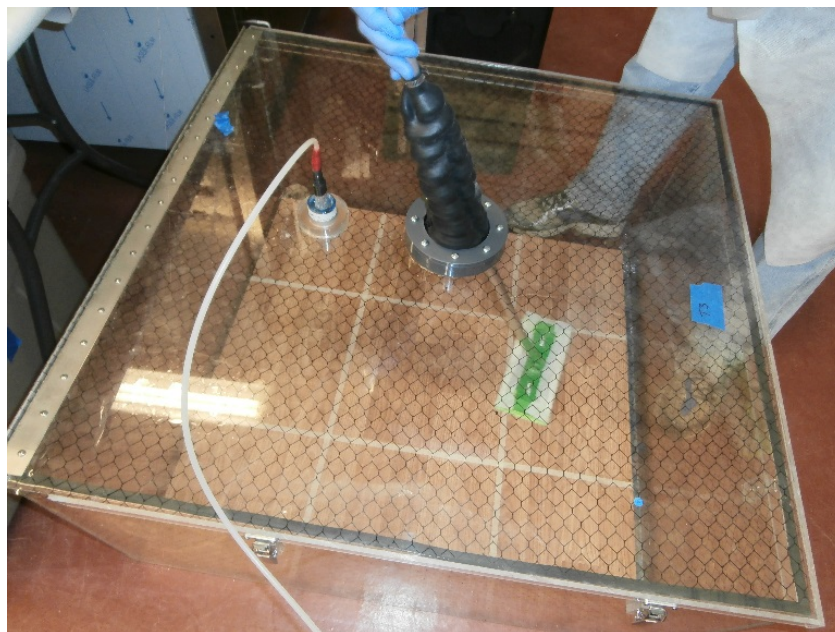
Figure 2-2: Laminate coupon located in acrylic testing chamber with Swiffer® and Via-Cell® ports
