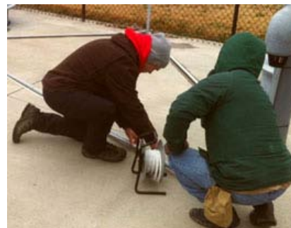
Laying out tubing for a sampling program.
