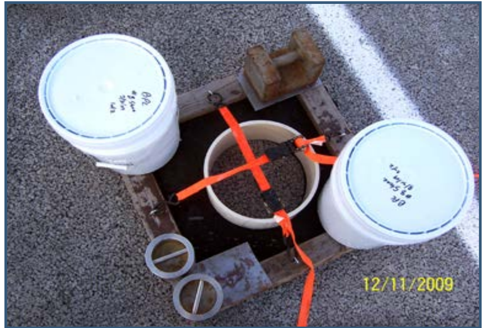
Modified ASTM C1701 apparatus
