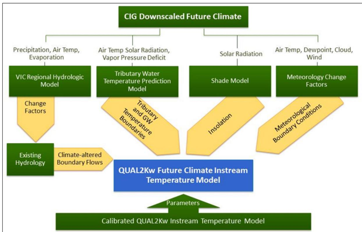
Figure 3-1. Schematic of Model and Climate Data Integration for the Quantitative Assessment
