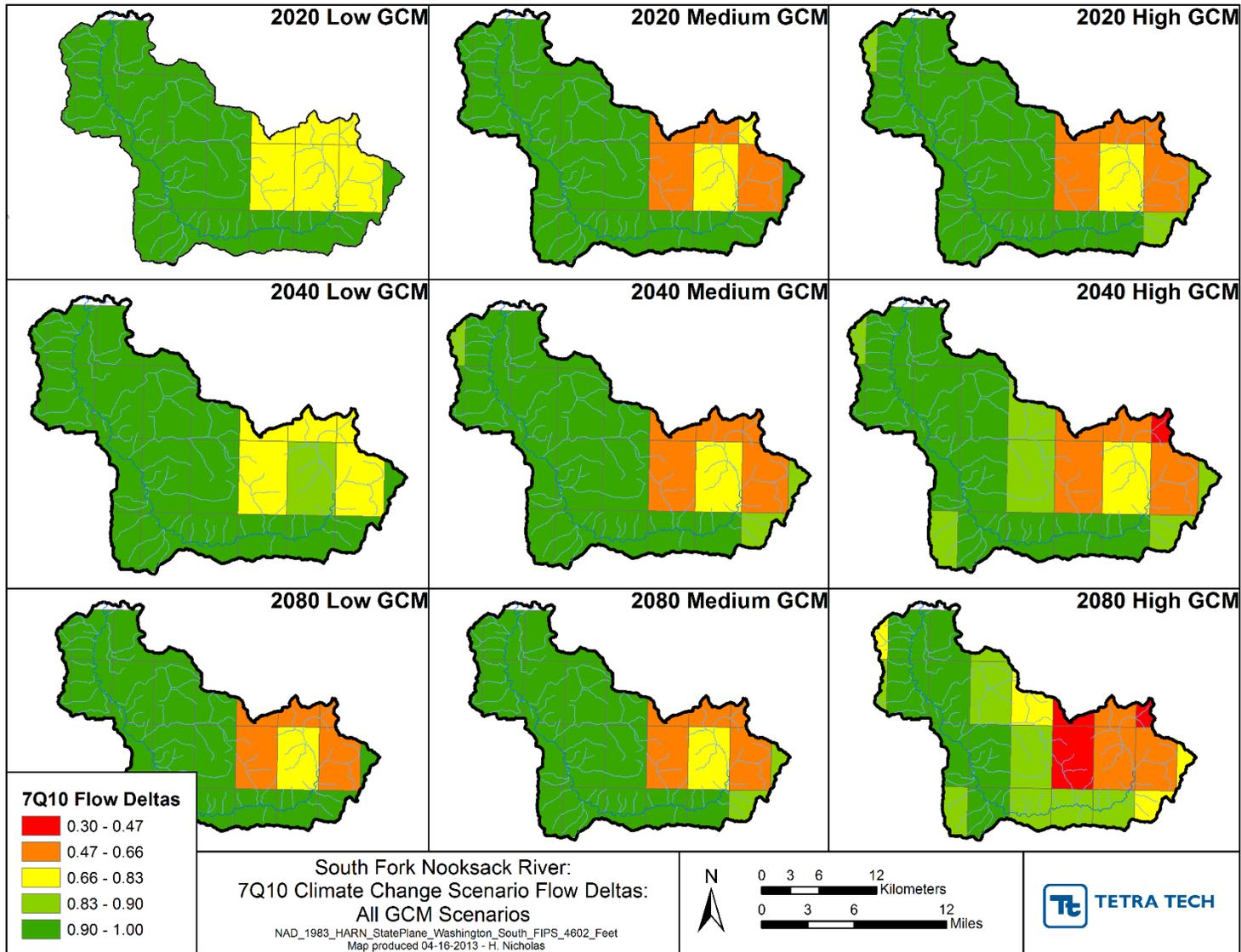
**Figure 4-1. 7Q10 Flow Multiplicative Change Factors (Unitless) for Tributary Flow from VIC Model for Low-, Medium-, and High-Impact Scenarios (Columns) and 2020s, 2040s, and 2080s Time Horizons (Rows)**
