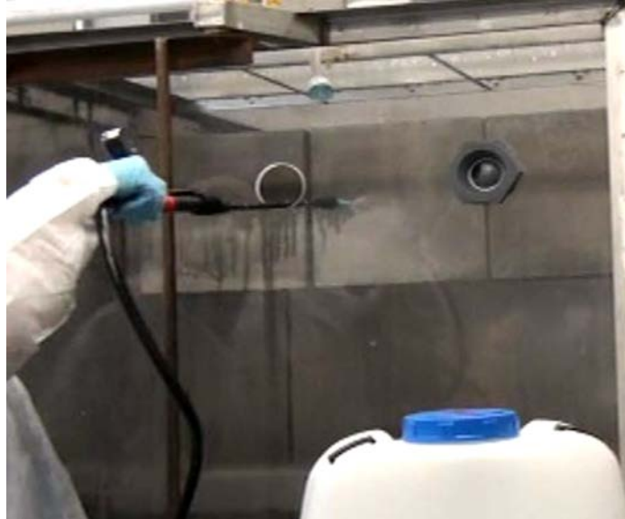
Figure 4.4-2. Spraying Through Center-Aligned Port in the Test Chamber Door
