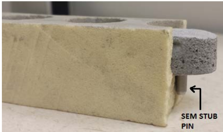
Figure 3.1-4. Cross Section of Final Small Concrete Coupon in Butterboard Mold
