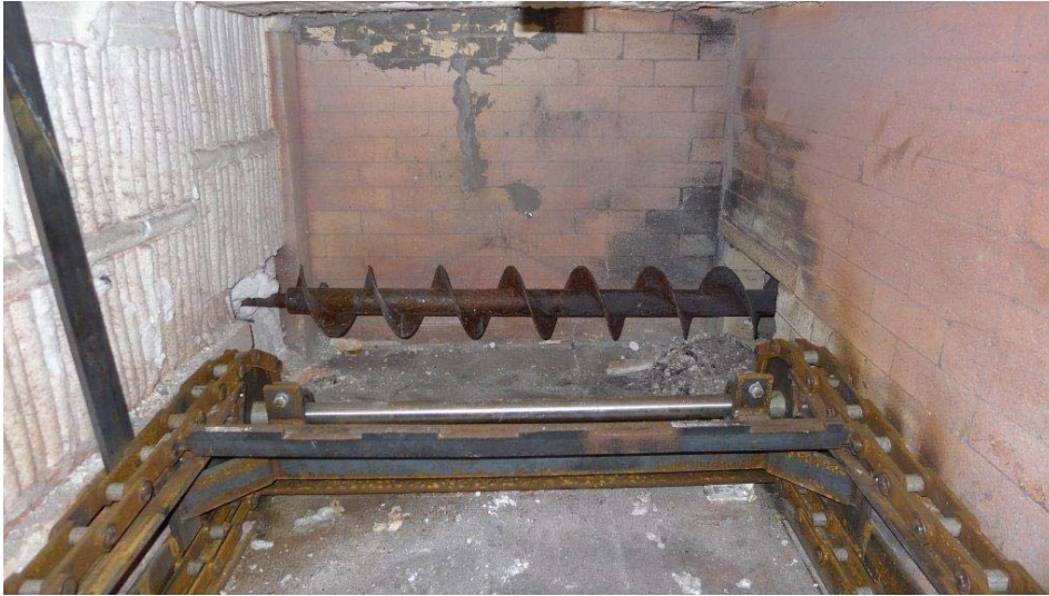
Figure 11. Gasifier Chamber showing Drag Chain and Ash Auger
