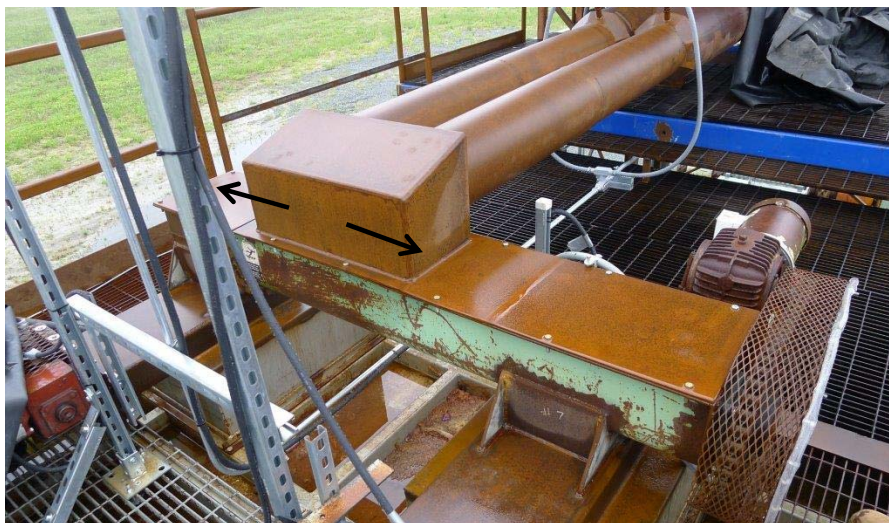
Figure 9. Screw with Opposing Flights to Gate Valves
