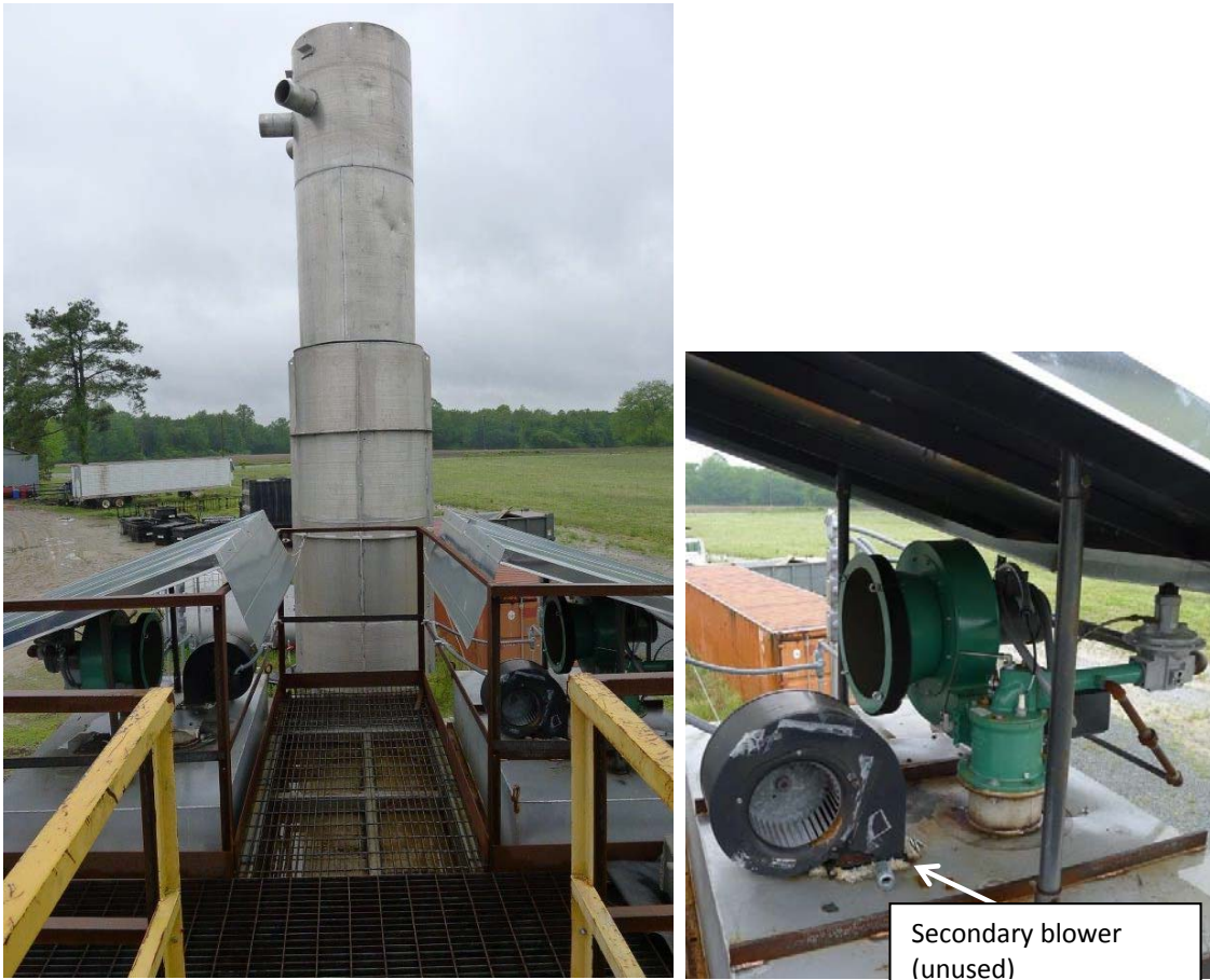
Figure 12. LP Burners and Exhaust Stack
