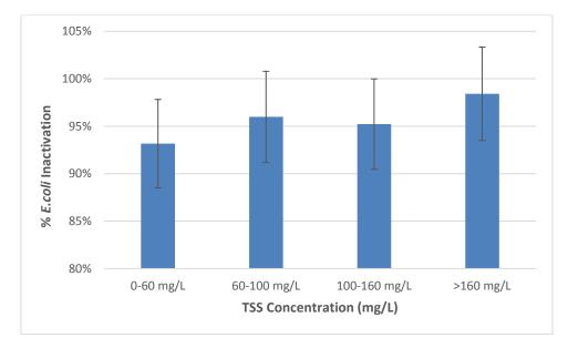
Figure 6: Percent inactivation of *E. coli* at 0-60, 60-100, 100-160 and >160 mg/L total suspended solids (TSS).
