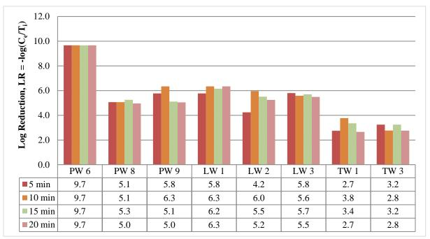
Figure 5: Log inactivation of *E. coli* at low flowrate (4 gpm or less) for tap water, pond water, and lagoon water (refer to Table 7 for definition of the samples).
