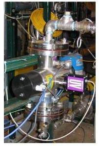
Figure 2: Medium pressure UV lamp system.
