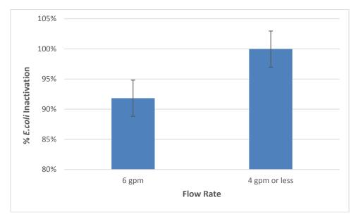
Figure 7: Percent inactivation of *E. coli* at high (6 gpm) and low (4 gpm or less) flow rates.
