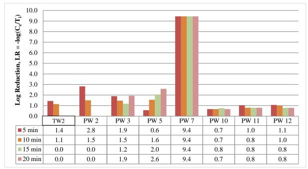
Figure 4: Log inactivation of *E. coli* at high flowrate (6 gpm) for tap water and pond water (refer to Table 7 for definition of the samples).
