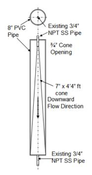
Figure 3: Cone diffuser used for ozone concentration with national pipe threat taper (NPT) stainless steel (SS) pipe.
