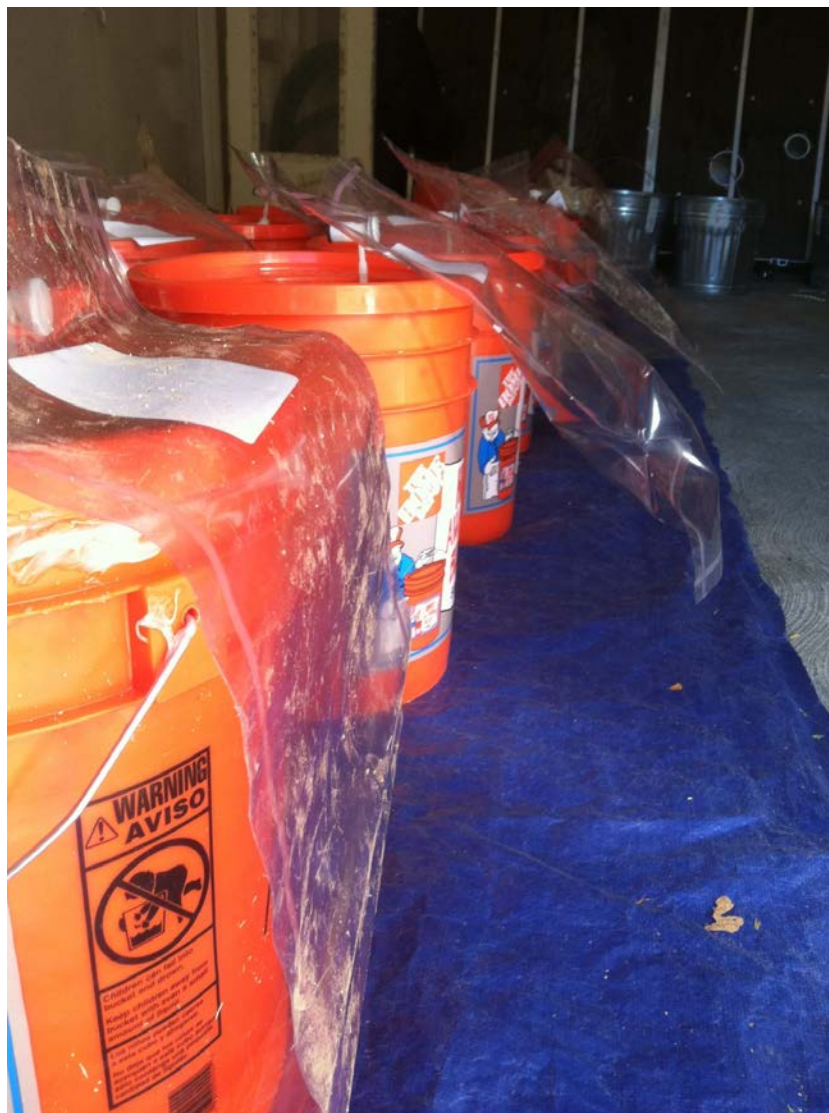
Figure 3. Gas collection bags directly attached to the mini-silos, with no gas in the nearest bag, but visible volumes in the two bags beyond.
