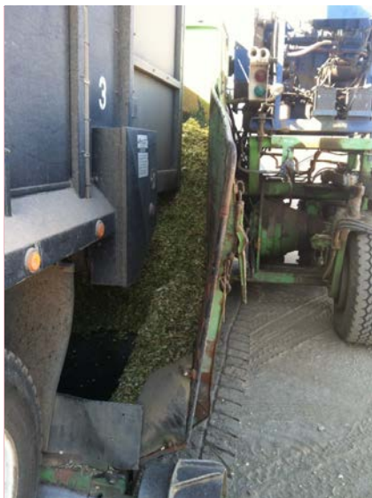
Figure 2. The open tray area for chopped corn collection, and the silage bags (white) being filled at the dairy.
