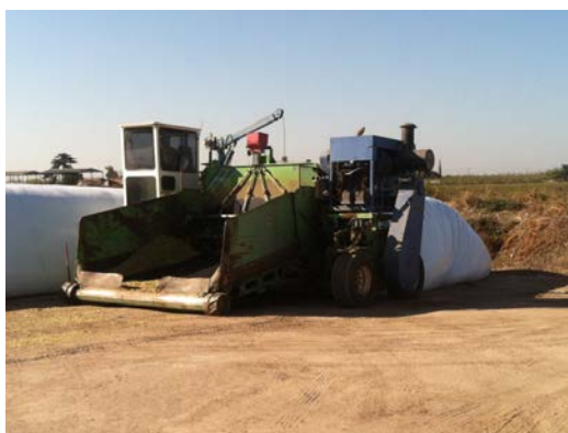
Figure 2. The open tray area for chopped corn collection, and the silage bags (white) being filled at the dairy.
