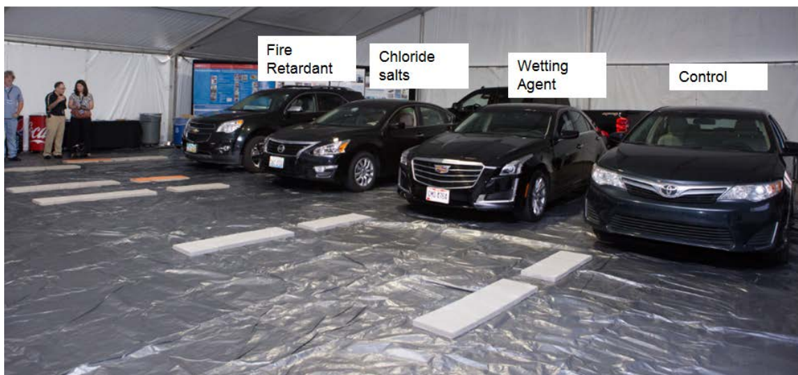
Figure 50. Vehicle orientation and associated containment technology for particle containment study.
