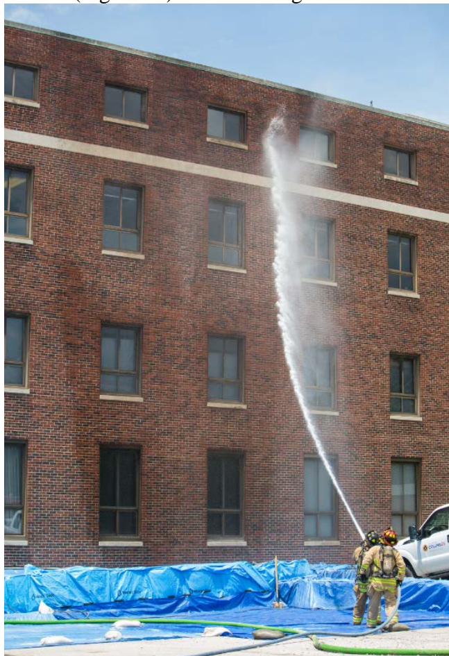
Figure 33. Application of water via a fire truck to simulate the IWATERS.
