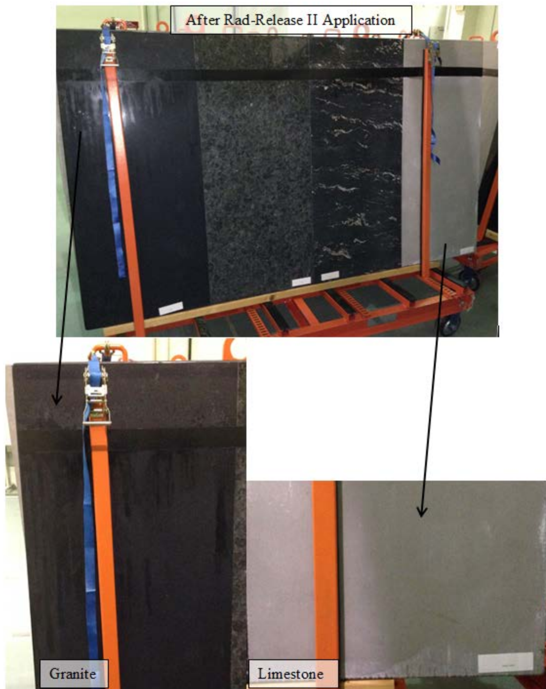
Figure 27. As seen in the images above, the condition of the granite and limestone changed after the application of Rad-Release II. The granite had a wet, streaky appearance, and the limestone showed white “chalky” residue. The appearance of the marble and quartz did not appear to be altered.
