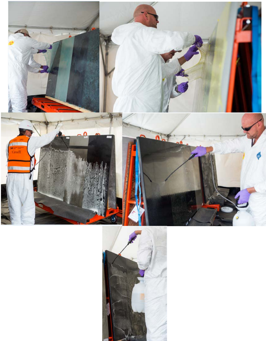
Figure 26. Removal of technologies from stand-alone surfaces. DeconGel (top left), Stripcoat (top right), UDF (middle left), Rad-Release II (middle right), SuperGel (bottom).
