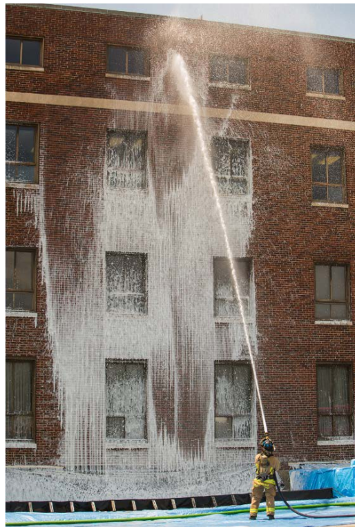
Figure 29. Water rinse to remove Environment Canada foam.
