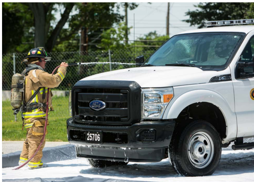
Figure 32. Water rinse to remove Environment Canada foam.
