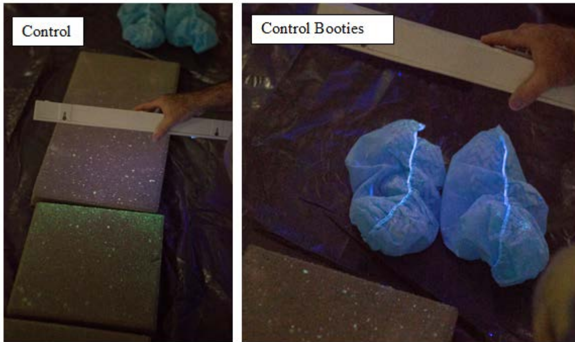
Figure 53. The image on the left shows control pavers and, as seen, the level of fluorescent particles on the pavers containing tracer is much greater than the pavers without tracer. The image on the right shows the booties worn in the control scenario after the demonstration was completed.
