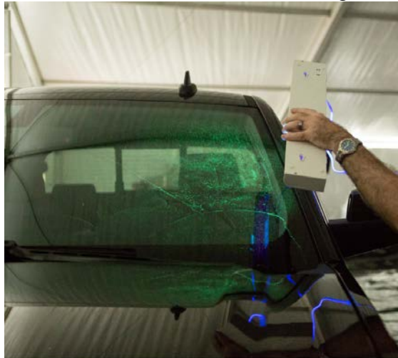
Figure 40. PDT-06 Simulation residue on the vehicle before the vehicle was washed.
