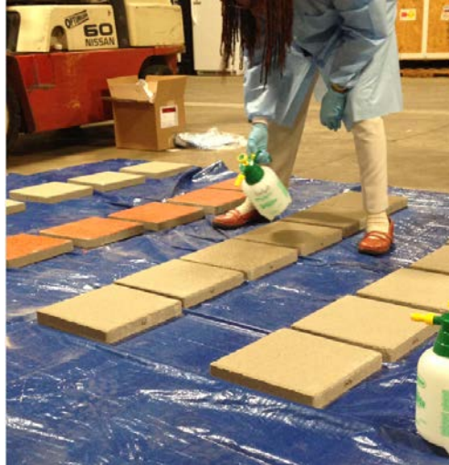
Figure 48. Application of containment technologies to pavers.
