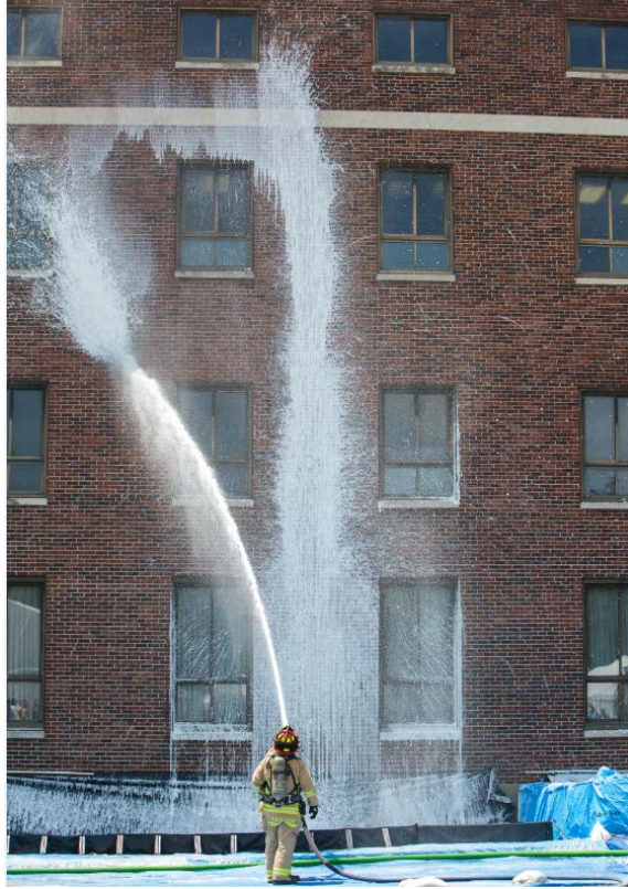
Figure 28. Application of Environment Canada foam via a fire truck.
