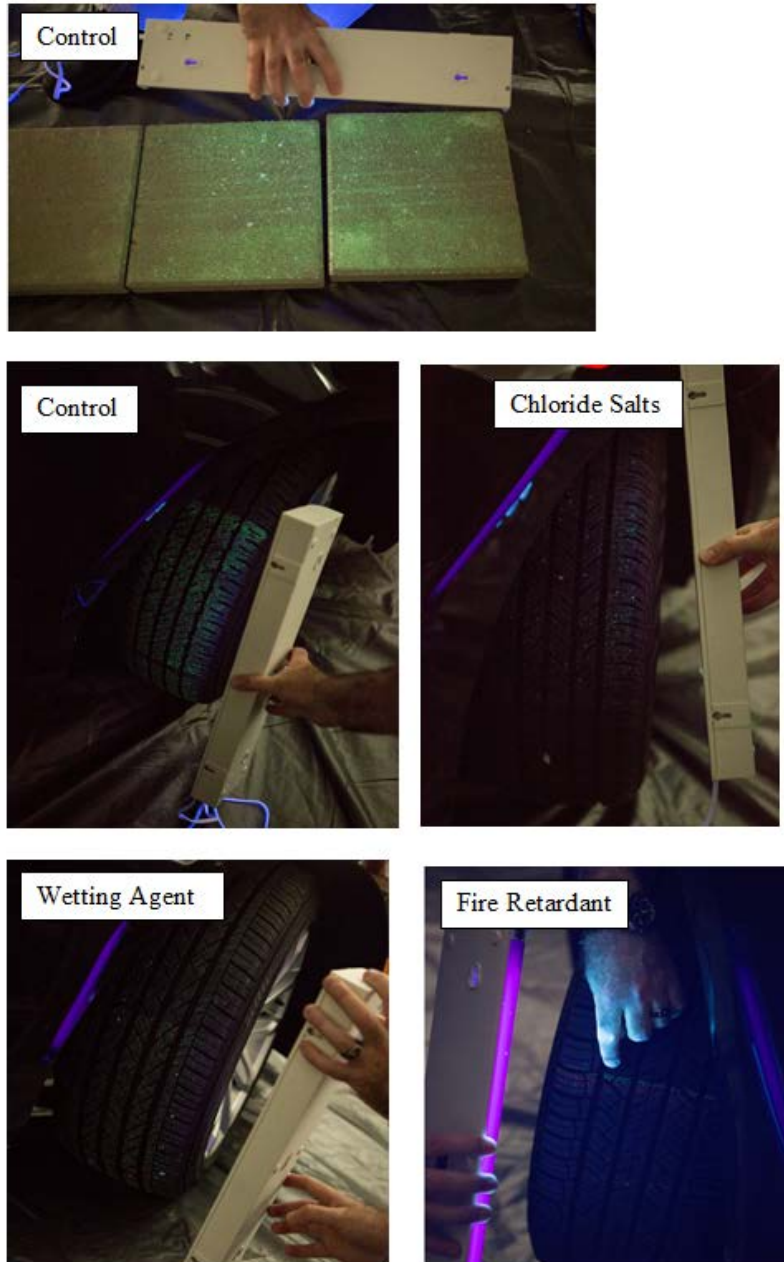
Figure 52. Results of the vehicle particle containment demonstration. Top image shows the control pavers after the vehicle had driven across. The control vehicle tires picked up the most particles (middle left), followed by the chloride salts. Wetting agents picked up a moderate number of particles (middle right and bottom left). The fire retardant scenario had the least amount of particle transfer (bottom right), but notice the narrow line of particles that was present when the tire contacted the edge of the paver, not covered by fire retardant.
