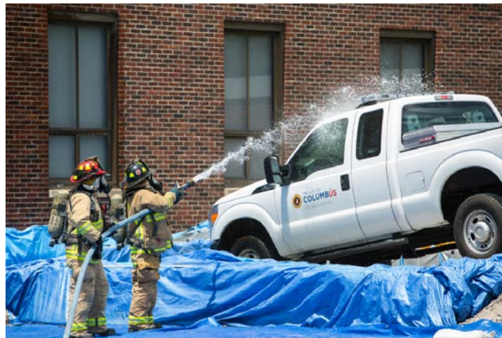
Figure 38. Vehicle wash occurring in HESCO ® berm to simulate IWATERS application.
