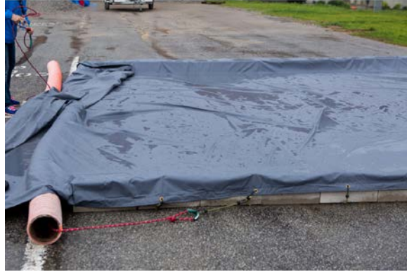
Figure 43. Image of the readily constructible containment berm.
