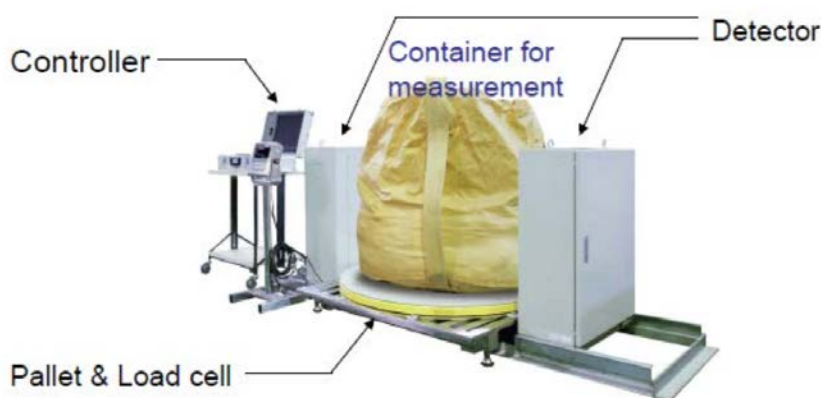
Figure 2-2. Toshiba's Simplified Method for Measuring Radioactivity Concentration per Container (MOE, 2013a)
