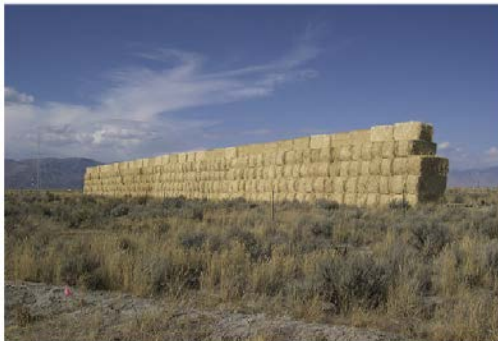
Fig. 1. Mock straw bale sound barrier, 6 m high and 90 m long.
